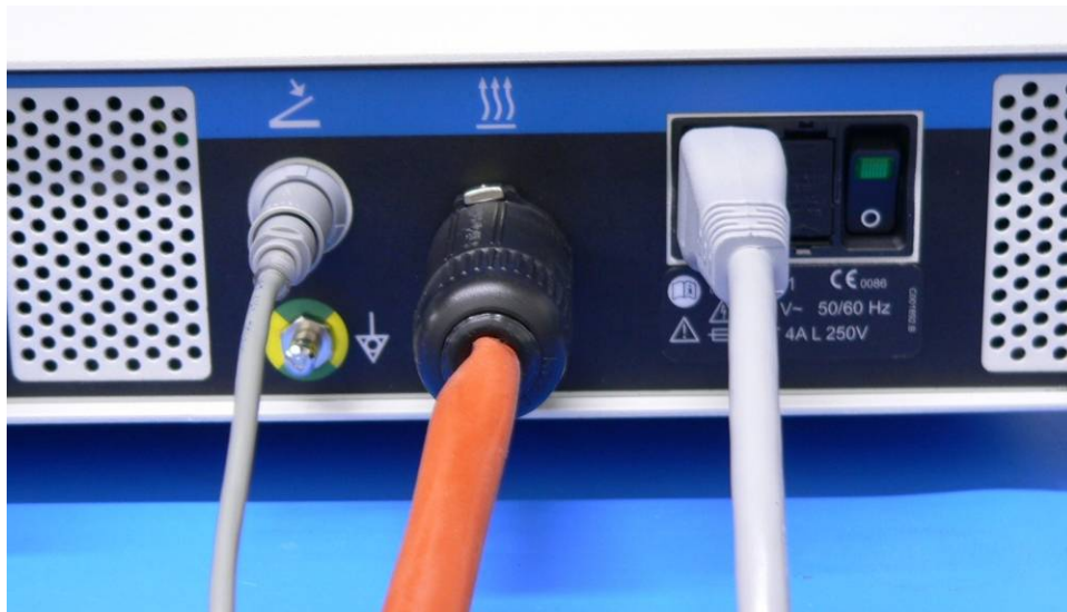
Figure 7 – Connecting the Footswitch, Cylinder Heater Band, and Power Cord to ACM
