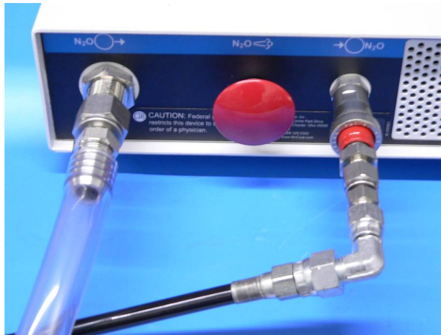
Figure 9 – Connecting the N 2 O gas line hose and N 2 O exhaust hose to the ACM
