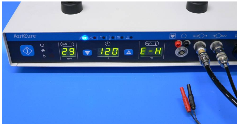
Figure 12A – ACM Indicating Missing Handpiece Thermocouple
