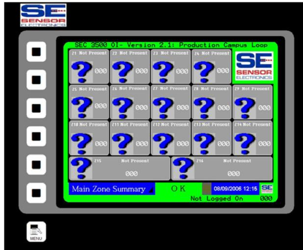
If so, then this is either the first time the 3500 has been powered on, or you do not have the Gas Monitoring loop setup/configured properly, or you have not detected any SEC 3500 compatible devices yet. Otherwise, if at least one compatible device is connected, online and had been setup previously, then at least one of the sixteen zone summary boxes would be green- see below:
