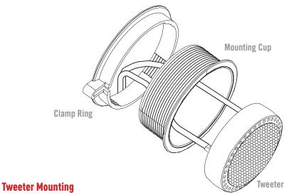
When flush or surface mounting tweeters, make sure the desired location can accommodate the hole size and depth required. Mount the cup using provided hardware (flush mount illustration shown on right.) Mount surface cup at desired angle with provided screws in tweeter mounting kit. Snake speaker wires through tweeter cup, connect tweeter to wires, and snap tweeter into cup by aligning the notches. Be careful not to push on the center of the tweeter grill.
