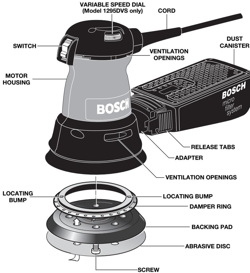
**⚠ CAUTION** To prevent possible swirl marks. Do not start the tool on the workpiece. Always run the tool for at least one minute before operation. This allows the tool to reach full speed.
