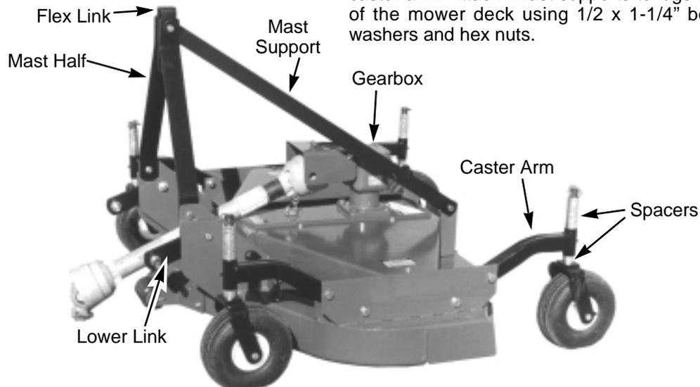
E. Fasten mast supports and upper flex link to mast halves using 1/2 x 5" bolt, pivot tube and locknut.
