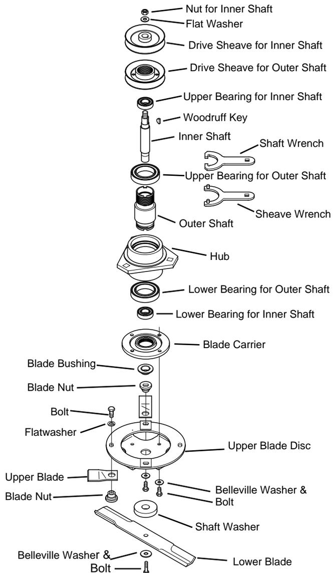
C. Thread the outer shaft sheave and blade carrier onto the assembly. **These threads are left handed - to tighten, turn counter-clockwise.** Clamp the blade carrier in a vise and insert the sheave wrench pins into the outer drive sheave. Using a torque wrench in conjunction with the sheave wrench, tighten the assembly to **200 ft./lbs.** Refer to Fig. 4-6 on following page for the required torque for your specific torque wrench.
