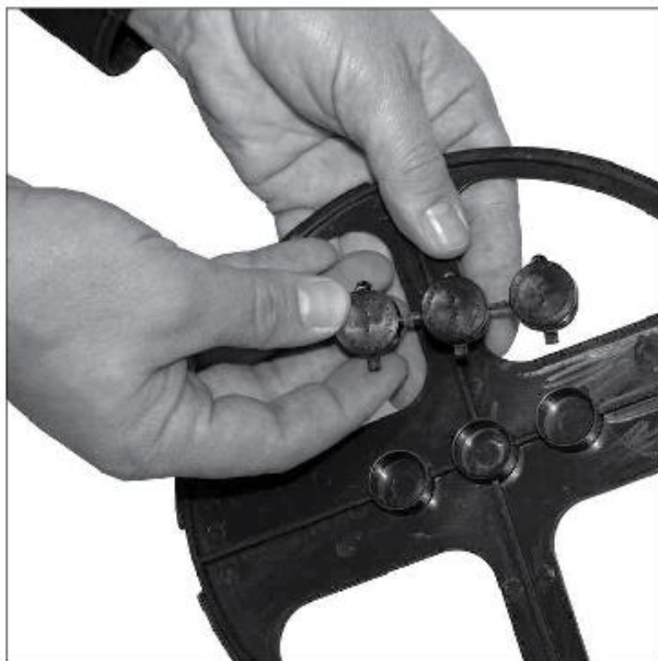
Fig. 3 Place the attractant cartridges in the dedicated holder on the bottom plate with pierced openings facing up.
