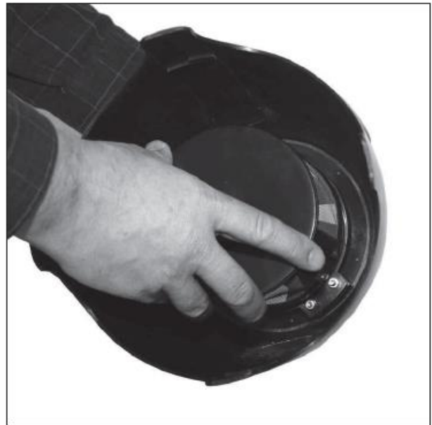
Fig. 4 To remove the catch container turn it anti clockwise.
