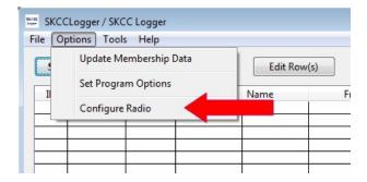
If you have a radio currently connected with an open COM port, you *must* first close the COM port before adding or editing any radio configurations. Close the COM port by pressing the "Close Port" button on the Radio Setup window.
