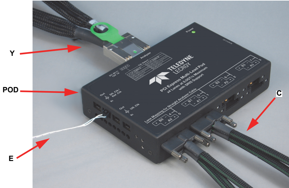
Figure 2: Teledyne LeCroy Gen3 Multi-lead Probe Pod and Components
