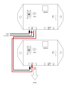
Note: When using a single device you can use the remaining 12VDC connector to power an external power relay (reference: KRT). Be sure that your power supply is sufficient (12V DC 1A is suitable)
