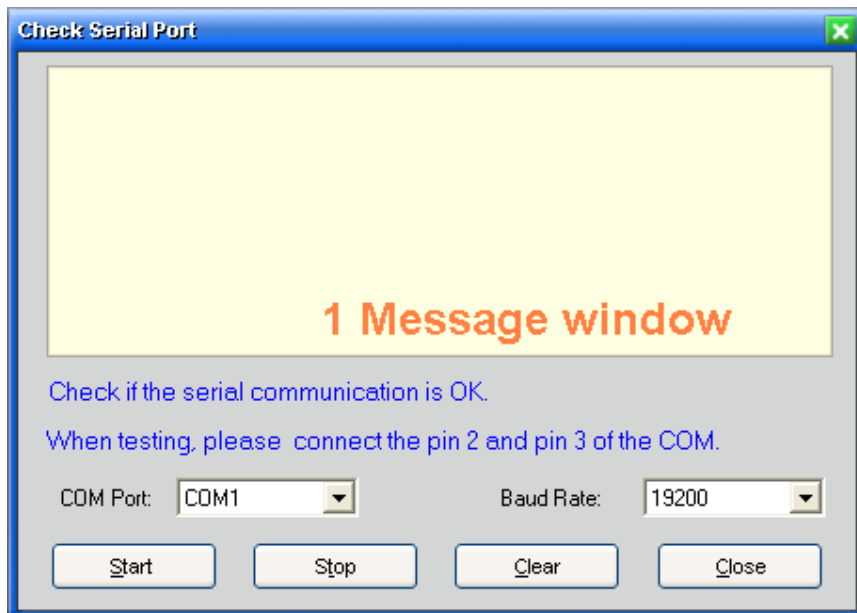
Fig. 6.14 Window of Checking a Serial Port
