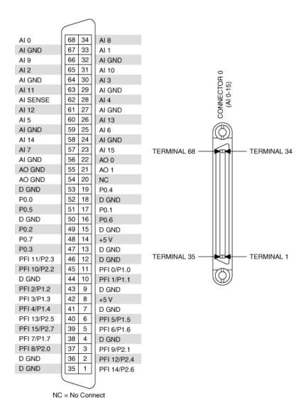
PCI/PXI-6221 (68-Pin) Pinout
