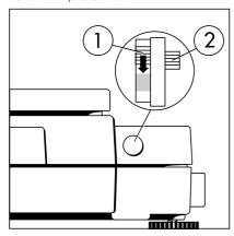
Switch up: external calibration blocked (factory setting on verified scales)
