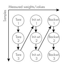
You can define the weighing sequence in the Setup menu or by pressing the Wa.sea (if the "Weighing sequence key" option is activated).
