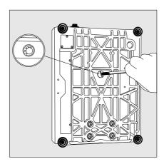
Fasten the hook to the cross-bar (see "Accessories").  If necessary, install a shield for protection against drafts
