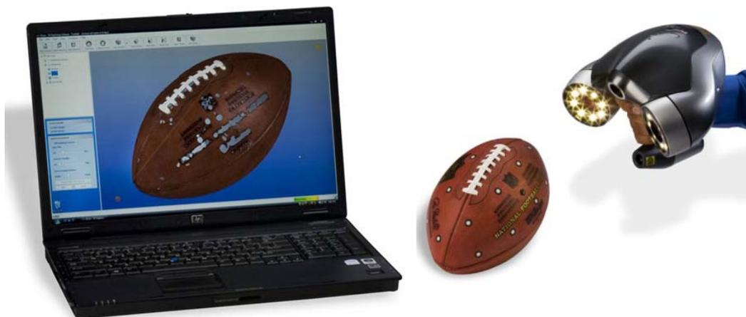
Figure: 1 – Real time scanning
