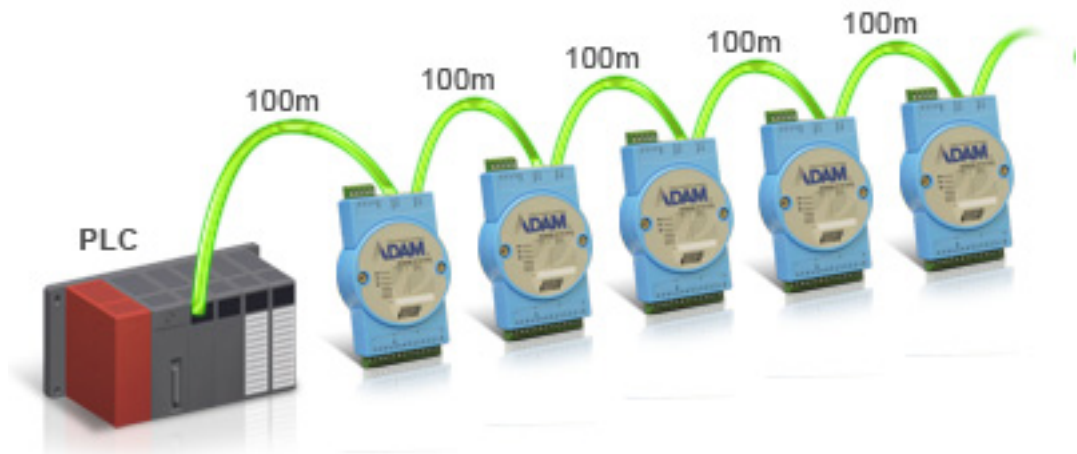
Figure 1.1 ADAM-6100EI Daisy Chain Connections
