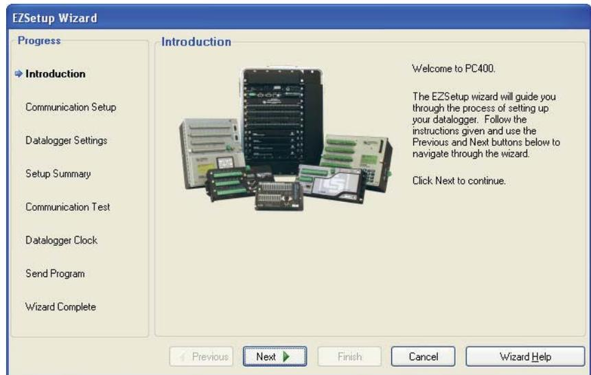
Previous and Next buttons are provided to move through the wizard. Progress is shown by the blue arrow next to each step displayed at the left. Help is available from the Help button as well as the text displayed on the right side of the screen itself.
