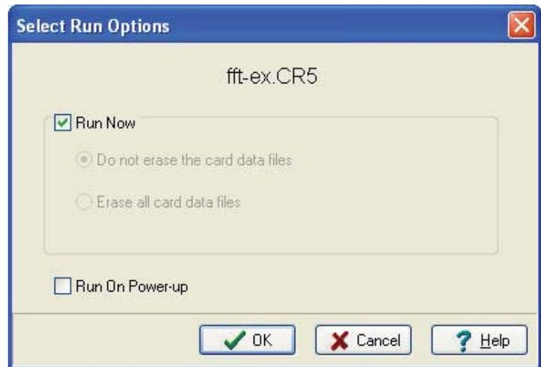
When Run Now is checked, the program is compiled and run in the datalogger. All data tables on the CPU are erased. You have the option of whether or not to erase data files stored on a card.
