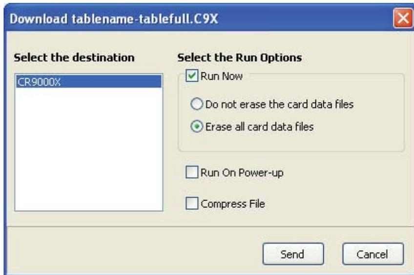
When Run Now is checked, the file will be sent with the Run Now attribute set. With this attribute, the program is compiled and run in the datalogger. All data tables on the CPU are erased. You have the option of whether or not to erase data files stored on a card.
