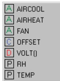
The variable list is sorted by variable type and then alphabetically by name. In the list above, the first green *A* denotes that the variable *AIRCOOL* is set up as an Alias.
