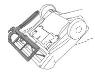
Remove brush assembly and check for wear on the belt.
