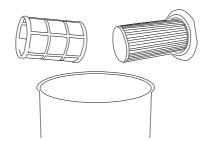
**IMPORTANT!** Ensure the mesh frame is reassembled to the filter before use
