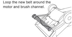
Hold the brush assembly and stretch the belt until the brush can be slotted back into the cleaner housing.
