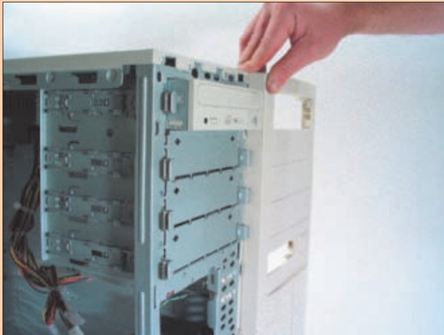
Figure 10-38 To judge how far to insert the optical drive in the bay, align it with the front of the case Courtesy: Course Technology/Cengage Learning
