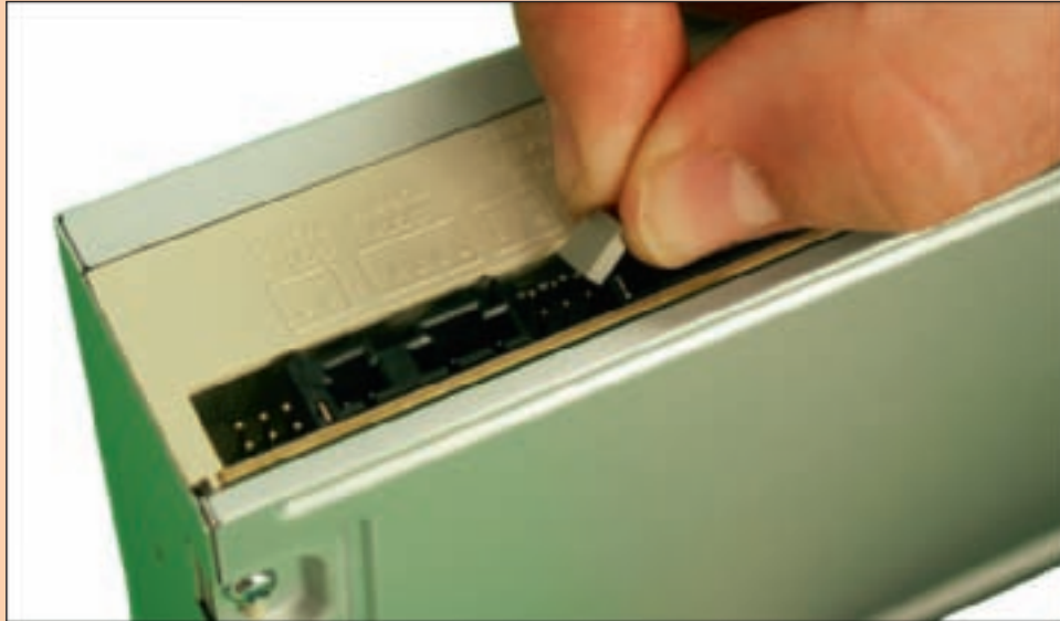
Figure 10-35 Set the jumper of an EIDE optical drive Courtesy: Course Technology/Cengage Learning
