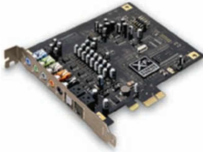
Figure 10-1 Sound Blaster X-Fi Titanium sound card by Creative uses a PCIe x1 slot Courtesy of Creative Technology Ltd.
