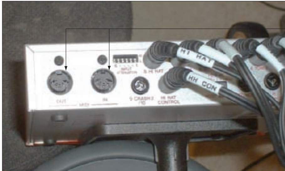
Figure 10-28 MIDI ports on an electronic drum set Courtesy: Course Technology/Cengage Learning
