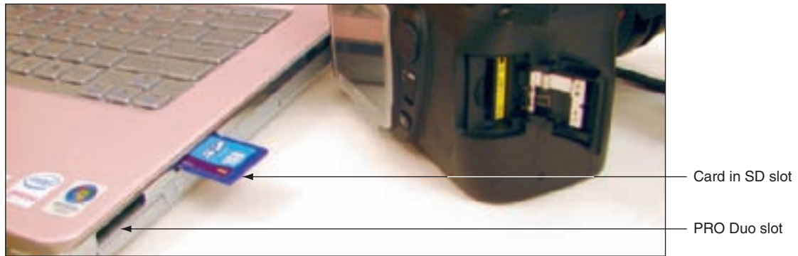
Figure 10-25 This laptop has two flash memory card slots Courtesy: Course Technology/Cengage Learning
