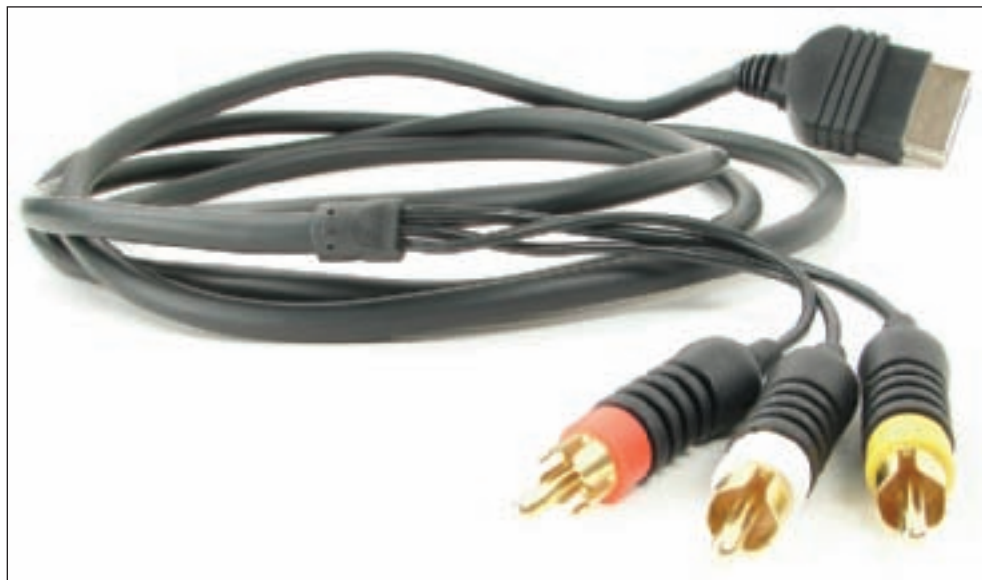
Figure 10-4 Standard RCA cable harness connects to game box Courtesy: Course Technology/Cengage Learning
