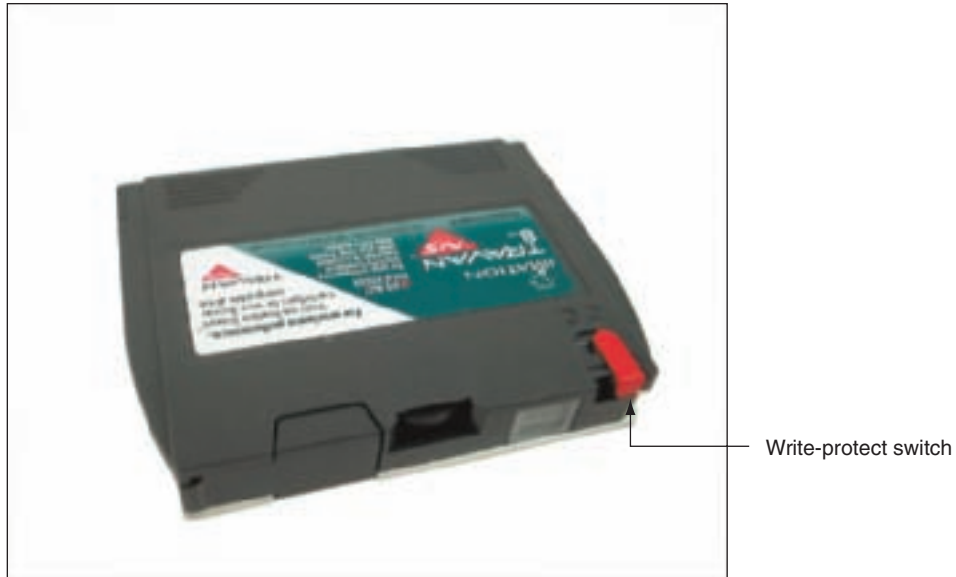
Figure 10-23 Minicartridge for a tape drive has a write-protect switch Courtesy: Course Technology/Cengage Learning
