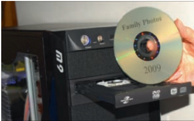
Figure 10-12 This disc label was written using a DVD burner that supports LightScribe Courtesy: Course Technology/Cengage Learning
