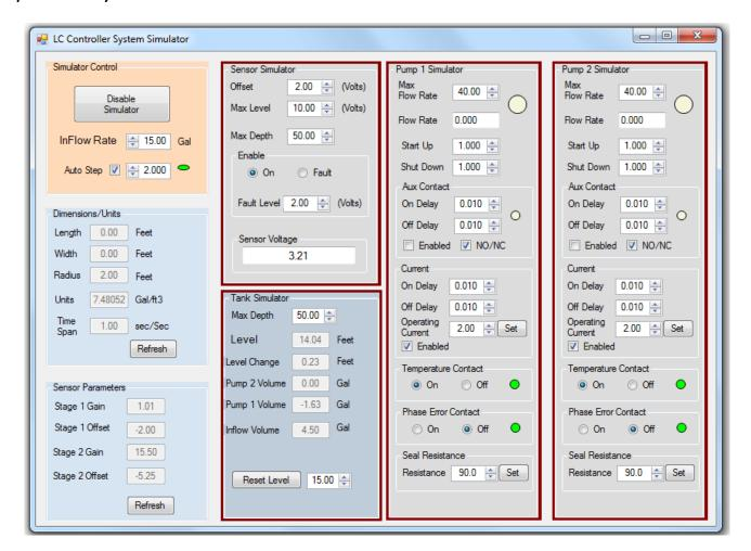
There are three major components to the Simulator: A Tank Simulator, a Sensor Simulator and 2 Pump Simulators. The simulator uses the parameters defined in the Level Detection subsystem (Sensor Data) and the Dimensions defined in the Flow Monitor subsystem (Dimensions, Time Span and Units).
