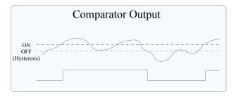
To avoid sporadic or false triggering a dual timer is used for each threshold that verifies the comparator output remains constant for a user defined time, referred to as the THRESHOLD ON and THRESHOLD OFF time. When the comparator is turned on it must remain on for the specified ON time. When it turns off it must remain off for the specified OFF time.
