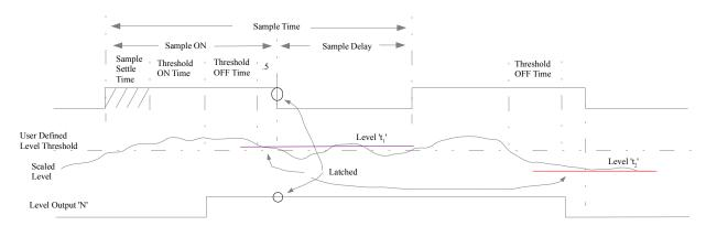
In Auto Tune Mode, the sample delay time is tuned by the system based on the user provided 'segment' value. Following a sample cycle, the change in level is compared to the current segment size and if the level has changed more than the segment size the Sample Delay is reduced. If the level has changed less than 1/2 of the segment size the Sample Delay is increased.
