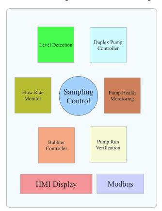
The LC-1 provides a fully functional Level Control solution in a small, DIN rail mounted controller. The integrated HMI provides access to an extensive set of run time statistics covering pump health, pump performance and system operating costs.
