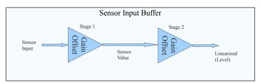
The LC controller accepts a 0-10 Vdc input, with an input impedance  $\gt$  50 Kohms. If a 4-20 mA sensor is used the signal may be converted to 2-10 Vdc using the following circuit. Stage 1 is typically used to remove the 2 volt offset by setting the Offset to -2.00 and the gain to 1.25, resulting in a Sensor Value signal of 0 - 10 Vdc.
