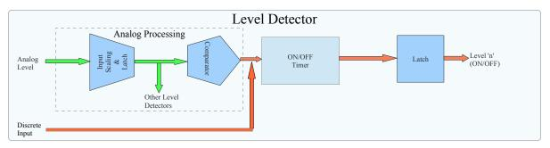
The Input Scaling and Latch function converts the input signal into standard engineering units (Feet/Inches or Meters/Centimeters), allowing user defined levels to be specified in the corresponding units, and then is applied to each level detector. In addition, the input signal is 'latched' as the current level during at the end of each sample period, allowing it to be used in the flow rate calculations.
