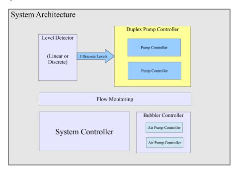
The Duplex Controller is implemented as 3 major components: a Pump Sequencer that selects which pump should operate and two Pump Controllers. Each Pump controller includes a Pump Health monitor that ensures the pump is capable of operating and a Run Verification monitor that ensures that the pump operates within specifications. In addition, several manual control functions are provided to allow enabling and controlling each pump as well as clearing error conditions and run time statistics.
