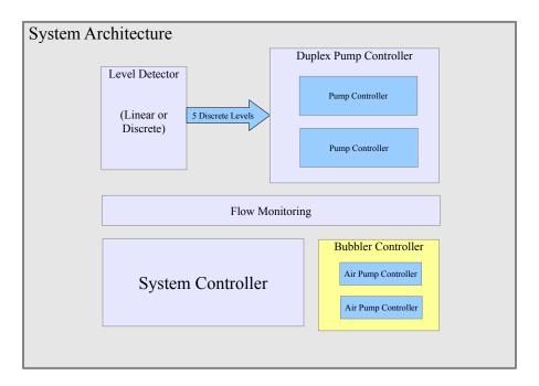
A Bubbler system measures the depth of a liquid by forcing bubbles up from the bottom. The air pressure required to force the bubbles is directly proportional to the depth of the liquid. A pressure transmitter connected in the air supply path may be connected to the Analog input of the Level Detector system to determine the depth of the liquid. A regulator is used to provide a constant air flow.
