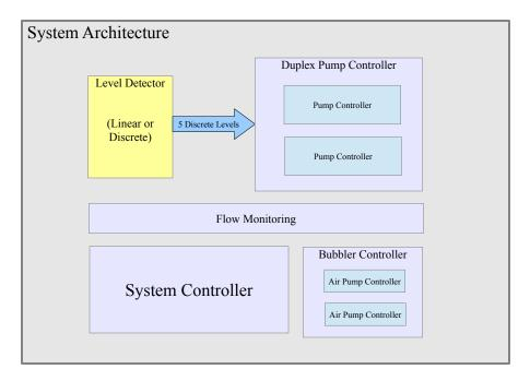
The level detection system supports 5 distinct levels. The linear level comparators include hysteresis to avoid false readings due to signal jitter. Following the threshold comparison the signal is further conditioned with a dual timer to ensure that the signal is stable prior to being latched at the end of each sampling period. Discrete level detectors apply the float signals directly to the dual timers.
