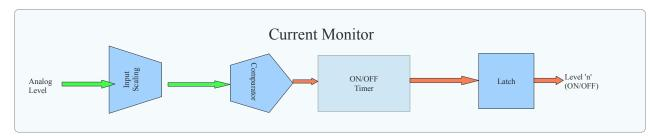
The Input Scaling converts the input signal into standard engineering units (Amps) allowing user defined levels to be specified in the corresponding threshold comparator. The Current Gain and Current Offset parameters allow converting the current sensor signal to 'Amps'.
