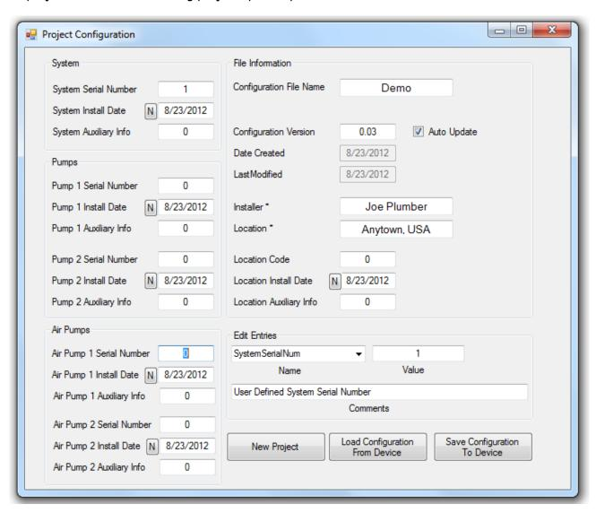
All of the fields entered are used as 'information only' fields and do not affect the operation of the LC controller. The information is stored as part of the configuration file as well as on the device.
