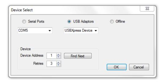
The Device Address must correspond to an LC device connected to the interface adapter. The default address is 1, although this may be changed using the LC HMI interface if several LC devices are connected to the same network.
