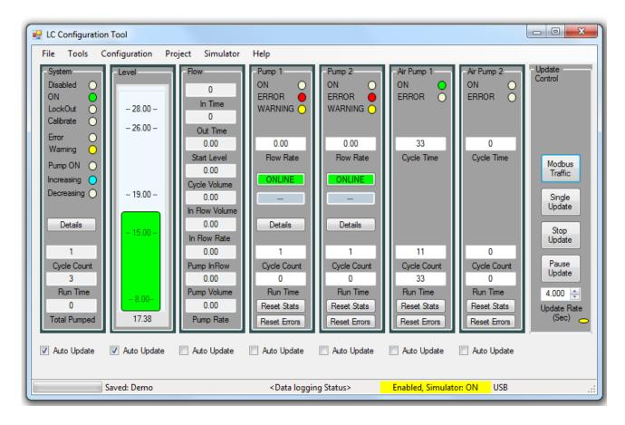
Each of the 5 major components of the LC controller (System, Level Detector, Duplex Controller, Flow Monitoring and Bubbler system) are represented by a number of 'control panels'. The Duplex Controller and Bubbler system each provide two panels, one for each of the pumps used within the subsystem.
