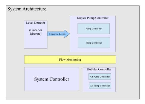
Flow rates are calculated by measuring the change in level over a unit of time and using the geometry of the holding tank to calculate the flow volume and flow rate. The system tracks the instantaneous level changes, the INFLOW rate and the estimated OUTFLOW rate.
