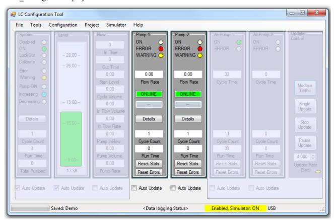
Additional Pump Details are available by selecting the 'Details' button on the appropriate Pump Control panel.
