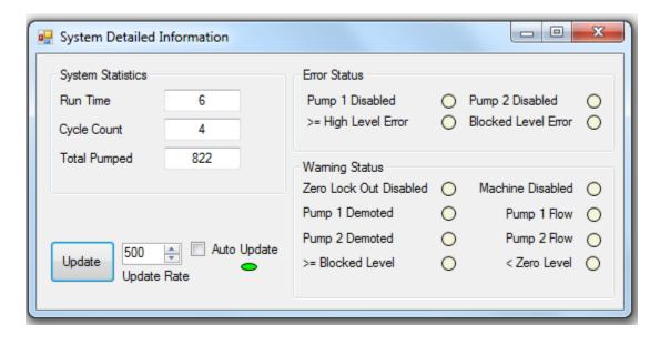
The Level Detector subsystem accepts either linear (analog) or discrete (digital) inputs and is responsible for determining the current level within the tank. A linear detector samples an Analog signal representing the current tank level which is compared against user defined setpoints. A discrete (float) detector accepts one of 5 digital inputs, typically connected to float switches, to determine the current level.
