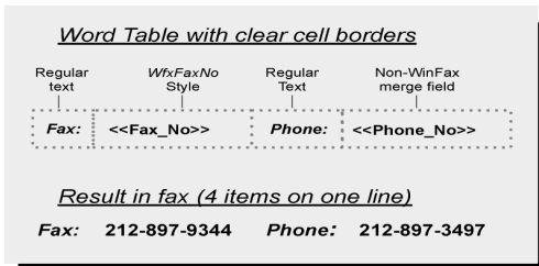
Figure 2. You can work around the “one-style-per-line” restriction by placing your elements in a Word table.
