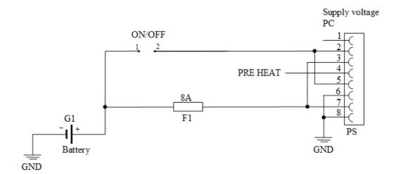
GND is connected to the vehicle's ground.
