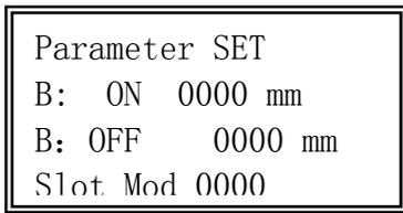
B ON 0000mm, Relay B, L<H switch output, L=0000mm
