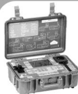
PAT-805 Portable appliance tester
