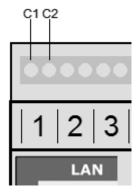
Connect the transducer for input 1 into C1 and C2 holes. For other inputs, use corresponding pairs of holes.
