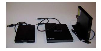
There are a number of options when it comes to getting information off of older computer hard drives. If you don't have a computer that supports the older drive, there are plenty of hard drive external enclosure kits available to interface all sizes of PATA and SATA hard drives to USB. The Apricorn DriveWire Universal Hard Drive Adapter is one of several similar products that can easily connect any size or type of bare hard drive to USB for data
