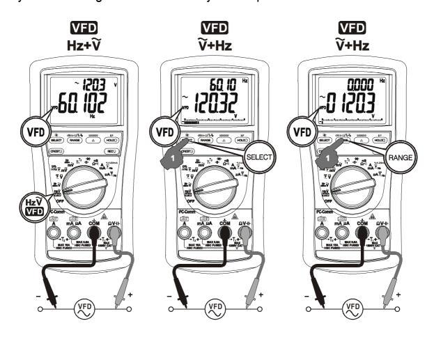
Note: Hz Input sensitivity varies automatically with voltage (current function alike) range selected. 5V range has the highest and the 1000V range has the lowest. This VFD
