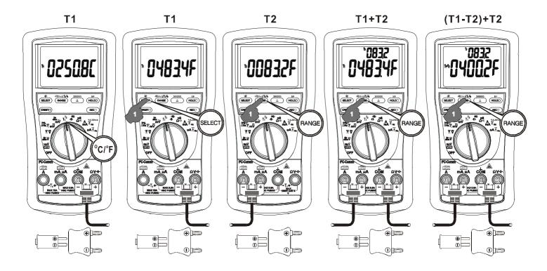
Note: Be sure to insert the banana plug type-K temperature bead probe Bkp60 with
