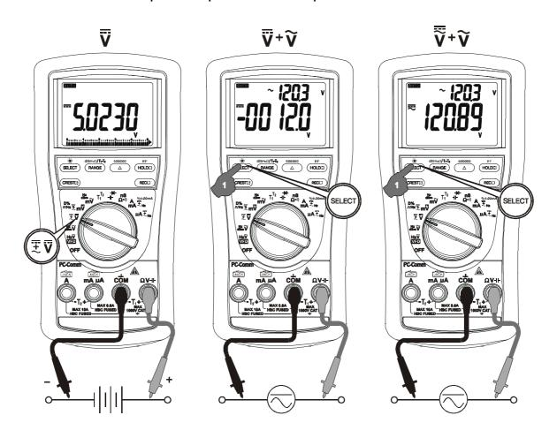
**DCmV**, **DCmV** +ACmV, **DC+ACmV** +ACmV, **Logic-Level ЛГHz**, **Duty% functions**Press the **SELECT** button momentarily to select the subject functions in sequence. Last selection will be saved as power up default for repeat measurement convenience.
