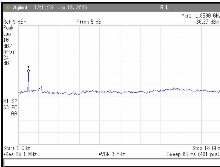
Plot 4. 802.11/b – Low Channel Conducted Emissions 1-18GHz
