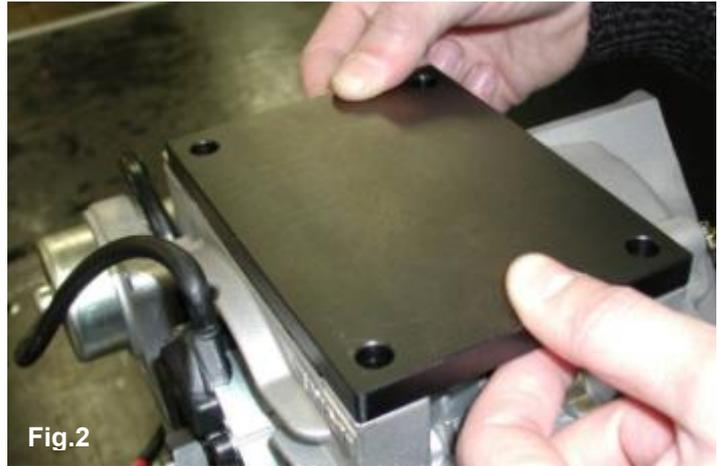
**3.4.3** INSTALL THE MOTOR MOUNT. MAKE SURE TO USE M8 ALLEN SCREWS WITH A LENGTH SUCH AS TO ENGAGE, IN THE CRANKCASE, A THREADED PORTION LENGTH OF 16÷19mm (THE SCREW MUST PROTRUDE FROM THE PLATE FOR 16÷19mm) (SEE FIG. 3 AND DRAW. PAG. 10)
