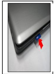
Hold the SD/MMC/MS card with its orientation symbol pointing into the slot and the topside of the card facing up.
