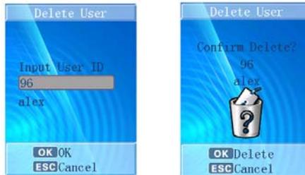
Input User Number, if the number is existed, it will be deleted; otherwise, that information: “User is not existed” will be shown on the screen and it will quit automatically. Press OK to confirm, “Confirm Delete?” will be displayed, and utter the hint voice, press OK again to delete the selected user.
