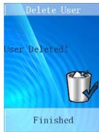
“User Deleted!” will be shown on the screen and the correct hint voice can be heard, the system will return to the “Delete User” menu automatically.
