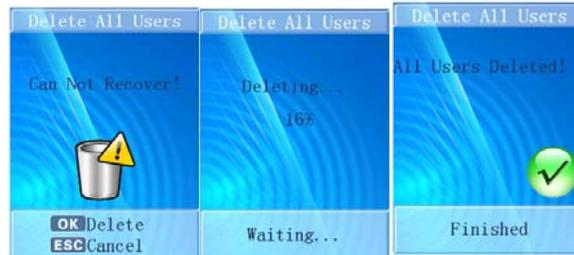
Press ESC to cancel and the system will return to “Delete User” menu. Press OK to start this function, all users’ information will be cleared and “Deleting...Waiting...” and rate of process will be displayed on the screen. After that, “Finished” will display and the correct hint voice can be heard, after 2 seconds, the system will return to “Delete all Users” menu automatically.
