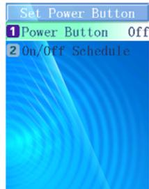
The power button can control the button in the keypad whether available. And device has an power on and off schedule. There are two time points can be set. One opening time and one closing time can
