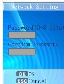
Press OK to confirm the setting, the complete networking information will be shown on the screen; it will utter the correct hint voice and restart the device automatically.
