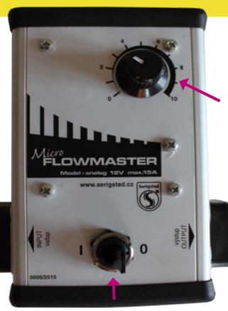
Controlling potentiom-eter setting up the pump capacity.
