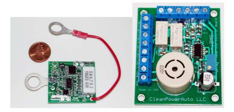
MiniBMS is a battery management system designed for LiFePo4 cells, used in Electric Vehicles. MiniBMS is designed to be reliable and cost effective solution; it has most basic functions, implemented via simple analog circuit and one wire interface, which also allows easy installation and troubleshooting.
