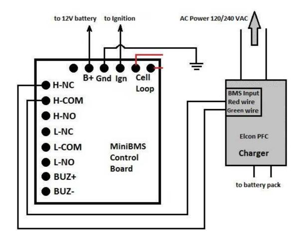
This diagram is for new style Elcon PFC charger with 7 pin round connector, which simply requires closure of Red/Green control wires to enable the charger. Some older variations may have Red/Black wires, which should work the same way.
