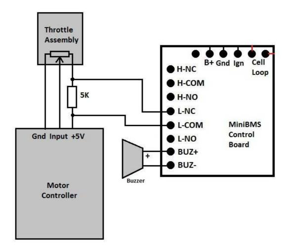
Next diagram shows only motor controller portion of MiniBMS wiring diagram for 3 wire Hall Effect throttle. Since Hall Effect device is powered by 5V input, we must use voltage divider on the output side of the throttle to reduce its output level during LVC event.
