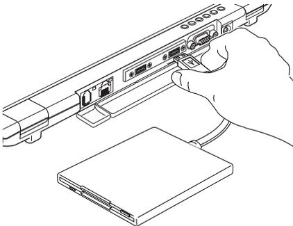
*Attaching the optional diskette drive cable to one of the computer's USB ports.*
