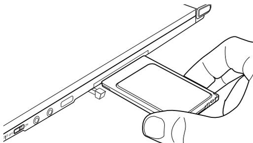
*Inserting a PC Card into the slot*
