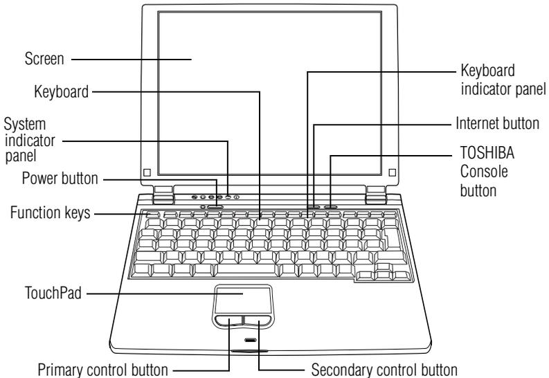
The computer's **screen** is a Poly-Silicon Technology, Thin Film Transistor (TFT), liquid crystal display (LCD) that provides clear, sharp, color images.
