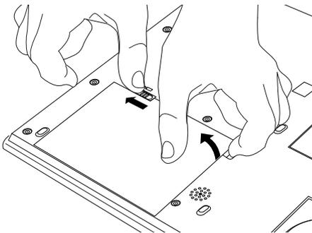
*Sliding the battery release latch and freeing the battery*
