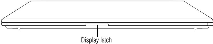
The **display latch** locks the display panel. Press the latch to release it.
