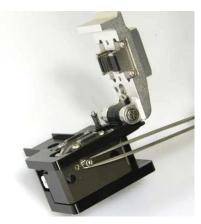
4) Be careful not to damage the blade. Assemble the part in the reverse manner. Tighten the set-screw firmly.
