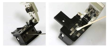
4) Turn the number on markings of blade by one click counterclockwise with a cotton swab. Fixing: reverse order.
