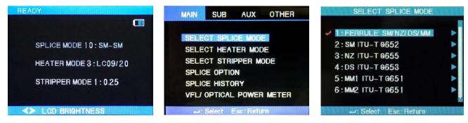
2) Use up or down key to move and select a splice mode by pressing ENTER key.
