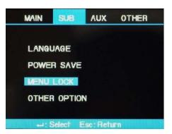
2) Select password and press ENTER key. Create a password by moving the cursor and press finish key to set or cancel the menu lock. If you select password locked, following items cannot be modified.
