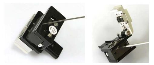
2) Adjust the blade height by turning Cam Pin with a flat-head screwdriver.
