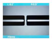
screen, check the condition of cross section through a naked eye inspection. Refer to below illustration. If one of below conditions is observed, remove the fiber from the equipment and place a new optical fiber. These conditions will cause a wrong splicing result.
