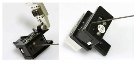
2) Insert a wrench into the hole at the bottom of the cleaver and loosen the Setscrew of the slider a little bit (about 2 turns). At this point, the slider has to be moved backward.
