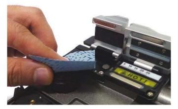
2) When the cleaner is used up and not discharged, open the cap and refill the cleaner. Cleaner is attached to OFS-920 body with a magnet so pull it up and completely separate it from OFS-920 body to refill the cleaner.
