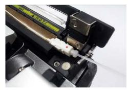
Heater Block-R assembly SC/FC/ST/LC Connector
