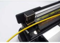
Heater Block-R assembly 250, 900, 2.0 ~ 4.0mm Indoor Cable
