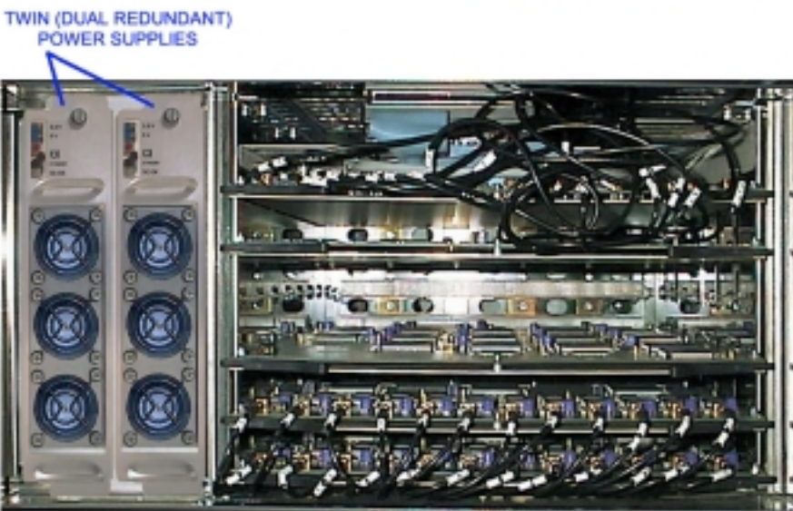
WITH TWIN POWER SUPPLIES USE BOTH POWER INPUT CONNECTORS
