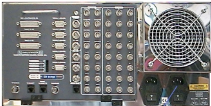
FOR SINGLE POWER SUPPLY SYSTEMS USE THE RIGHT HAND POWER INLET
