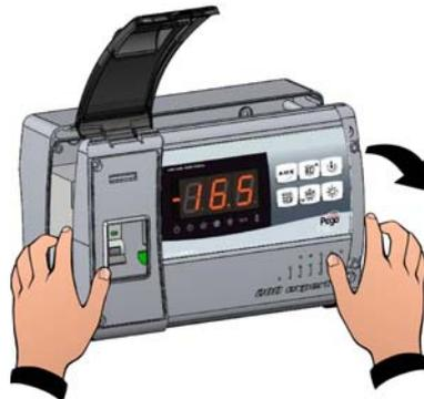
**Fig. 5:** Apply pressure on the sides of each hinge to release and fully remove the front.
