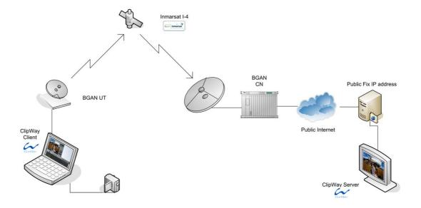
The solution consists of a server side software application which is kept at the studio, and a software encoder which can be loaded onto a laptop (at the client side). Connect the camera to the software encoder using a firewire cable. Connect the laptop to the BGAN terminal using any standard interface, such as Ethernet (recommended), USB and WiFi.
