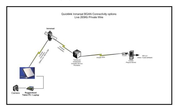
The solution consists of a decoder box which is kept at the studio, and a software encoder which can be loaded onto a laptop (at the client side). Connect the camera to the software encoder using a firewire cable. Connect the laptop to the BGAN terminal using any standard interface, such as Ethernet (recommended), USB and WiFi.
