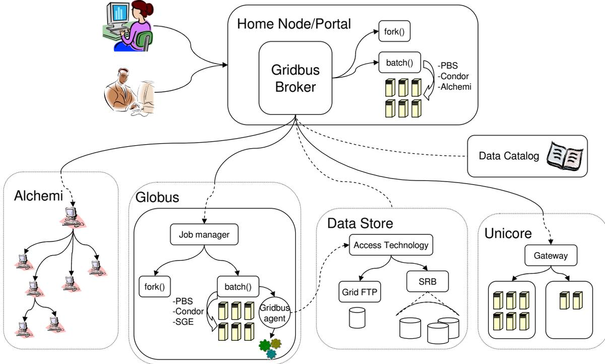
The Gridbus broker works with middleware such as Globus, UNICORE, Alchemi; JobManagers such as Condor, PBS; Data catalogs and also Data storage systems such as the Replica Catalog and SRB .
