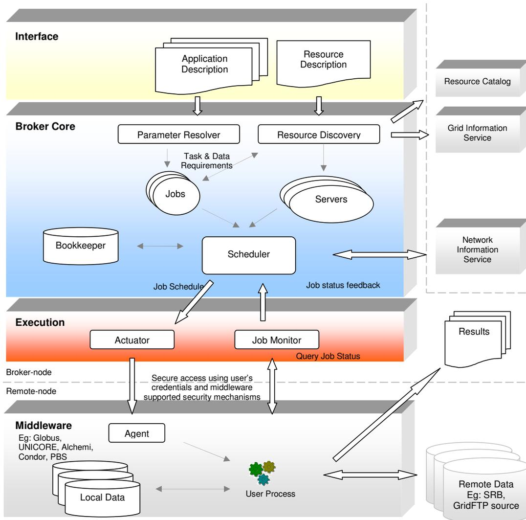
Figure 2: Broker Architecture
