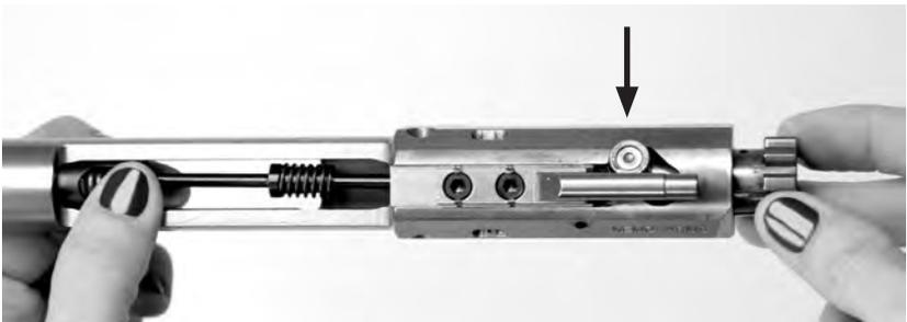
9 Remove the cam pin. Cam pin must be perfectly aligned in slot for removal.
