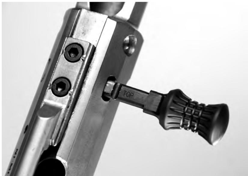
**Additional Lubricant** - Add two drops of CLP to the bolt cam pin slot, one drop to the entrance of the gas key hole. Lubricate the running surface on the bolt carrier with a higher viscosity lubricant or grease. The running surface on the bolt carrier is where the carrier touches and rides the upper receiver.
