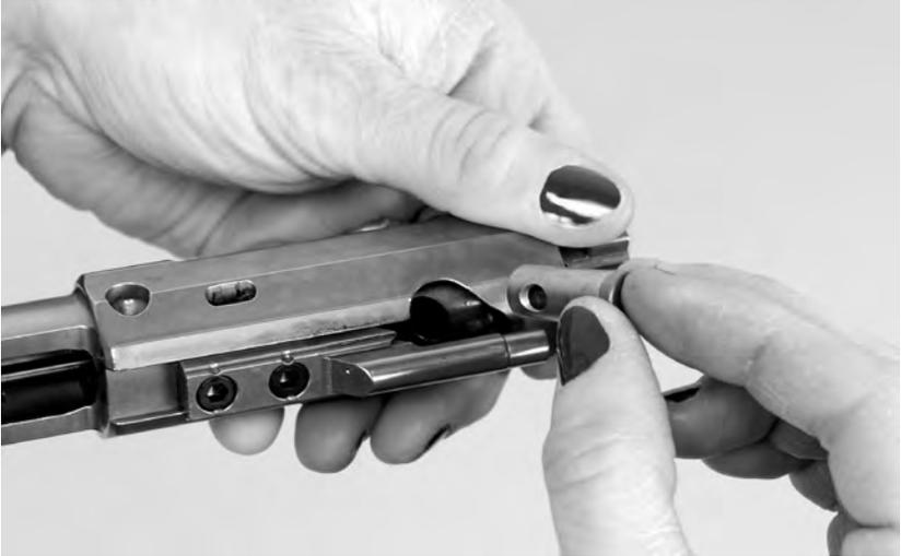
10 After cam pin is removed, pull bolt out from the bolt carrier
