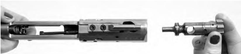
11 After the bolt is removed, pull out and remove firing pin. Pin can be removed from the bottom or the top of the slot.
