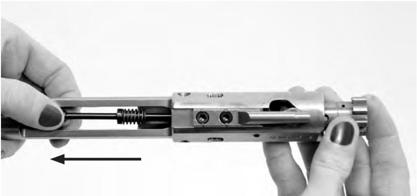
8 While holding the firing pin back, push bolt in and line up cam pin so that it can be removed. It must be able to clear the gas key.
