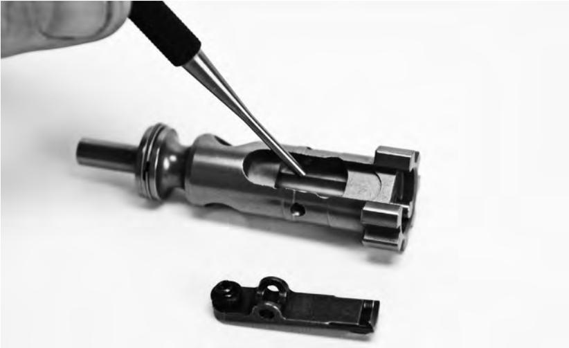
Your bolt carrier group is now completely field stripped for cleaning.
