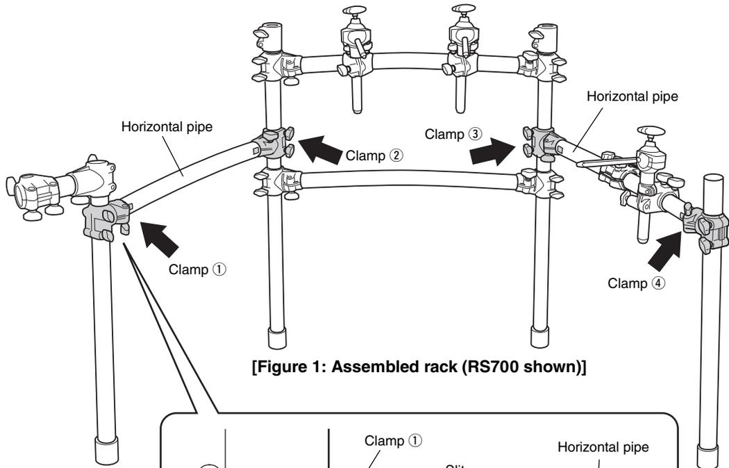
[Figure 1: Assembled rack (RS700 shown)]
