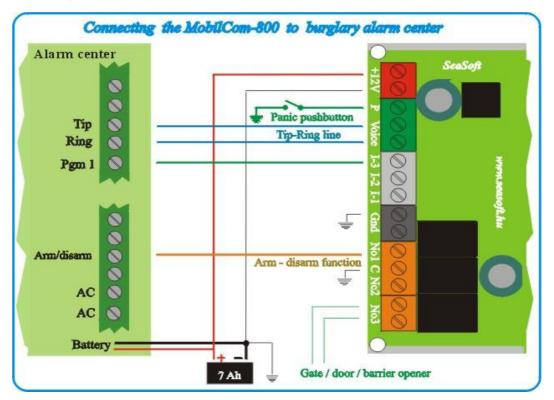
Connection of **MobilCom-800** panel to the alarm center has to be done according to the illustration. Connecting the power supply and **Tip-Ring** inputs is necessary while the panic input, remote arm or disarm and GSM gate-opener functions can be connected optionally.
