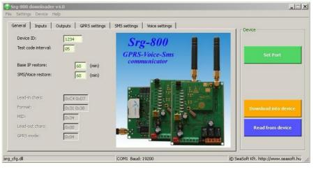
After this step it has to identify which serial port is connected to the device. It's possible the use the autodetect function or it can be found manually too. For example to do it this way in Windows XP: Control Panel -> System -> Hardware -> Devices and Printers -> Ports (Com)
