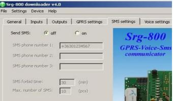
sending disabled. The secondary (SMS-based) transmission works only for the first number, the other numbers are for the remote controlling of relay outputs. The dialer discards every call from unregistered numbers and the GPRS transmitter forwards every Sms from unknown phone numbers
