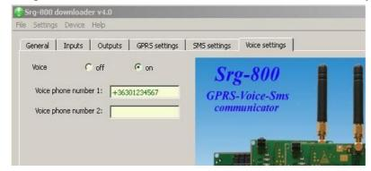
to the no. 1 SMS number and it does the same with SMS messages from the provider. In the Voice Settings menu the secondary transmission will be forwarded to the Voice 1 phone number. You can give two phone numbers in the **Voice Settings**, the first has to be the provider's primary number with international format, with + prefix
