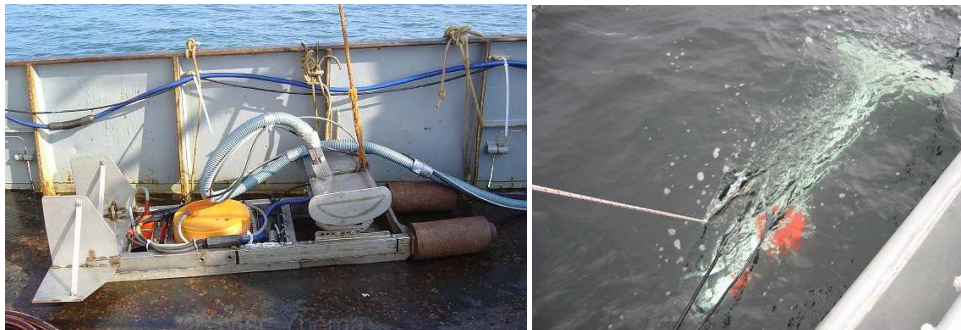
Figure 4.2. Towed body as used by FRS Aberdeen and IMARES (left panel) and image of a typical towing depth (right panel).
