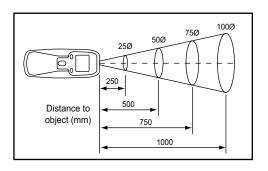
surroundings. Remember that the measurement size is one-tenth the distance to the target. For example, if the thermometer is at 10", then the size measured is 1".
