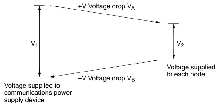
$V_1$ : Voltage supplied to the communications power supply device. Consider the ambient variations of the power supply voltage and take  $V_1$  to be 23 V.
