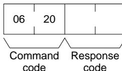
The response format is as follows when the parameter is 01 (when reading):
