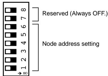
Pins 1 through 6 represent binary digits which are 1 when the pin is ON, 0 when the pin is OFF. Any node address from 0 through 63 can be set as long as it hasn't been set on another node (Slave).
