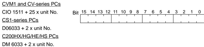
The current communications cycle time is stored in the above word as 4-digit BCD in ms. The value is truncated at the decimal point. The value is refreshed each PC execution cycle for CS1-series and C200HX/HG/HE/HS PCs and each peripheral servicing time for CVM1 and CV-series PCs.
