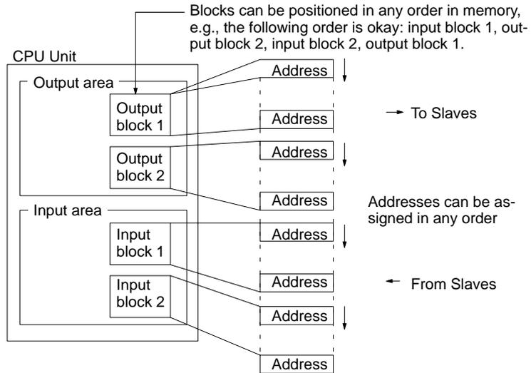
Allocation Methods and System Configurations
