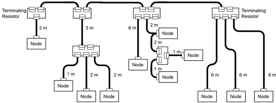
In the configuration example, the length of each drop line is 6 m or less as demanded but the total sum length of all the drop lines is 40 m. Set the baud rate at 250 kbps or 125 kbps because the total maximum length of drop lines at 500 kbps must not exceed 39 m.
