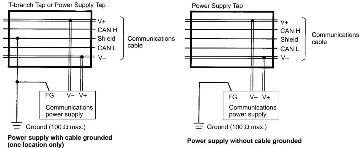
If more than one communications power supply is connected to the same network, ground only the one nearest the center of the network. Do not connect the shield wire at the other power supplies. Always use Power Supply Taps when connecting more than one communications power supply to the same network. (The power supplies are not counted as network nodes.)
