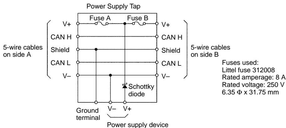
Remove fuse A when disconnecting cables on side A, and fuse B when disconnecting cables on side B.
