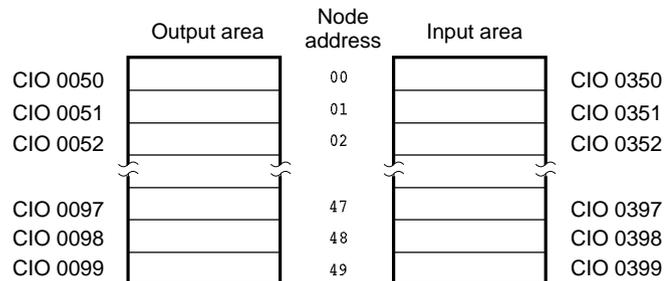
With the CS1 Series, the DeviceNet Output Area (CIO 0050 to CIO 0099) is contained inside the I/O Area (CIO 0000 to CIO 0319). For this reason, in systems with a large number of I/O points, where CIO 0050 to CIO 0099 would be allocated to I/O Units, ensure that there is no overlap of area allocation using one of the following methods.
