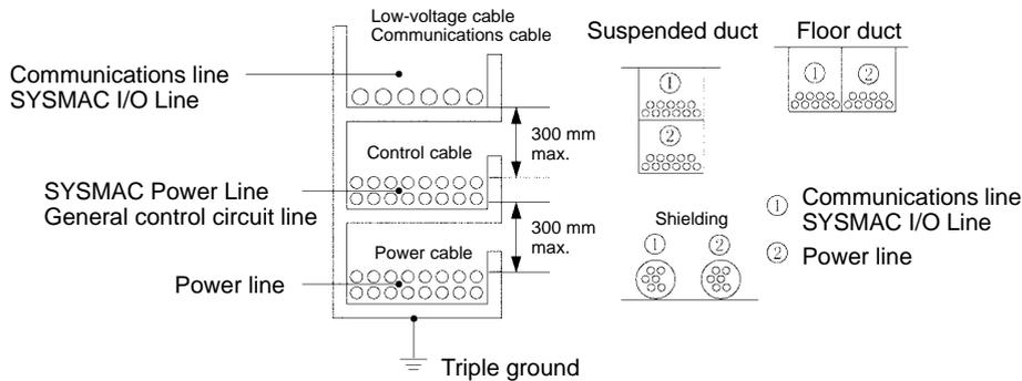
Do not install communications lines and SYSMAC Power Lines onto the control panel on which high-voltage devices are mounted.
