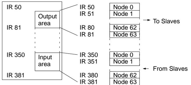
**Note** With the CS1 Series, the DeviceNet Output Area (CIO 0050 to CIO 0099) is contained inside the I/O Area (CIO 0000 to CIO 0319). For this reason, in systems with a large number of I/O points, edit the I/O table with the CX-programmer so that there is no overlap of area allocation.
