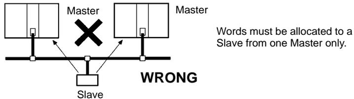
You can use the master parameter file duplication check from the Configurator to check for node address that have been set more than once in the scan list, which shows the I/O allocations that have been made.
