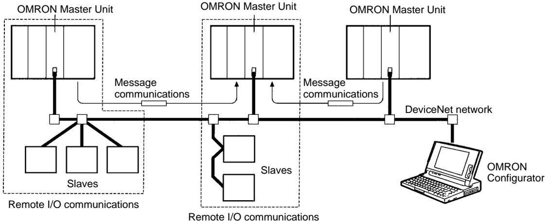
**Handles Multi-point Control and Line Expansions with Multi-layer Networks**
