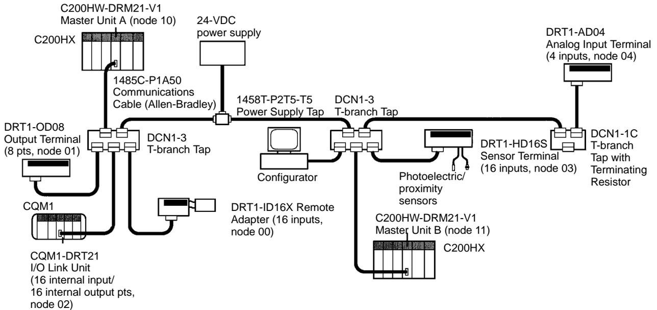
The following remote I/O configuration will be used for the above Network.
