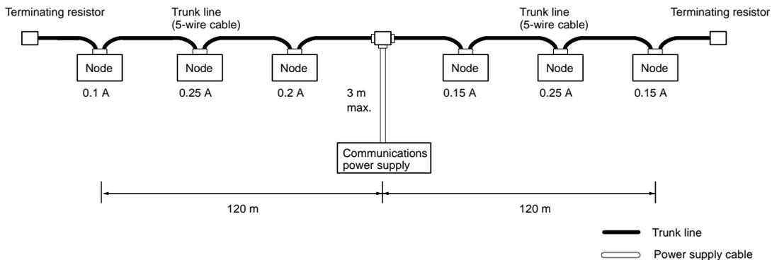
Total power supply length on left = Total power supply length on right = 120 m
