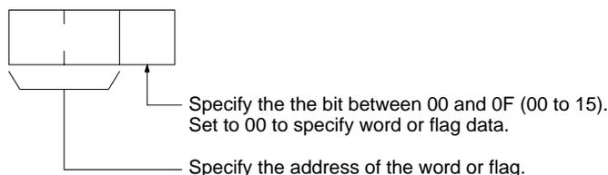
To obtain the corresponding address of the desired word or bit, add the data area word address (hexadecimal) to the first address of the range of addresses used for that data area in communications. For example, the address for word AR 13 is computed as follows:
