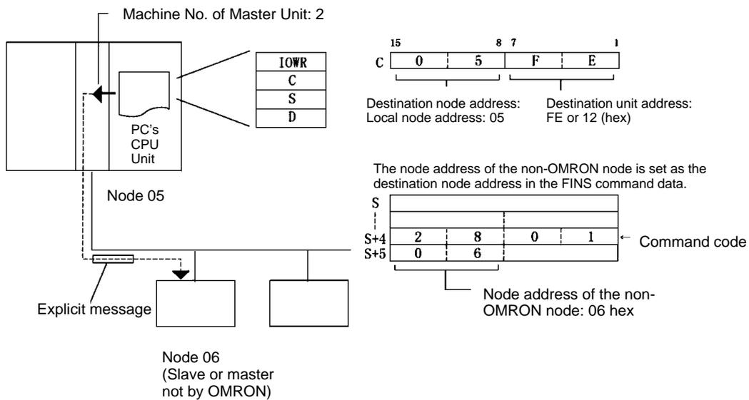
**Note** Explicit messages are first sent to the the DeviceNet Master Unit, which processes them before sending the actual explicit message to the final destination. You must use the node and unit address of the local Master Unit in the PC user program communications instruction. Addressing them to any other node will result in an error, such as would occur in the following illustration.
