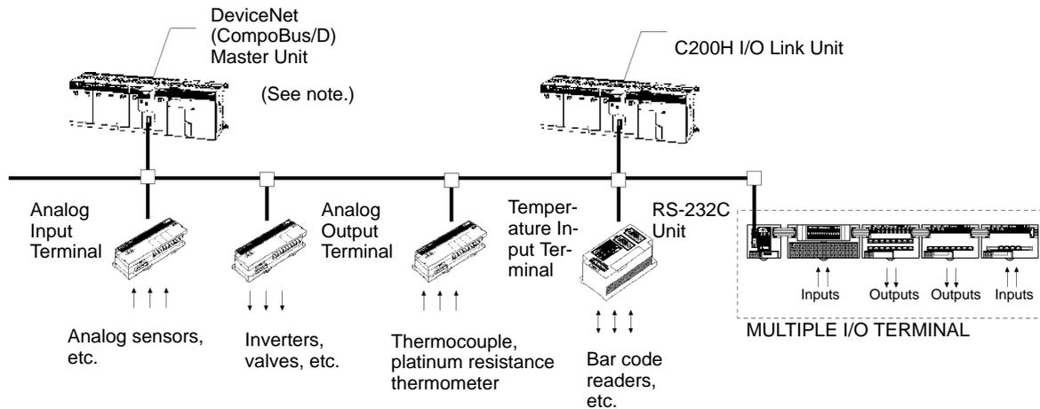
**Note** A Configurator is required for networks with more than one Master.
