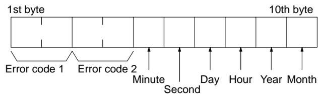
**Error code 1, 2:** Refer to page 184 for error code 1 and to the relevant operation manual or installation guide for error code 2.
