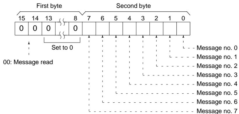
**Message (response):** Each message is read in the numerical order according to the message number. Each message consists of 32 ASCII characters (32 bytes). The total number of bytes of the messages is calculated as follows:
