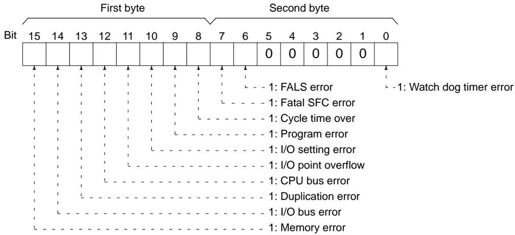
**Non-fatal error data (response):** The contents of PC non-fatal error information (for details refer to the *CV-series PC Operation Manual: Ladder Diagrams*):
