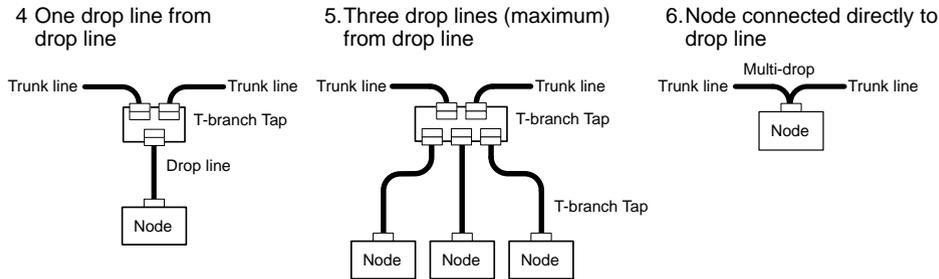
Various different forms of connection can be used on the same network, as shown in the following diagram. Any number of nodes up to 63 can be connected onto a single drop line.
