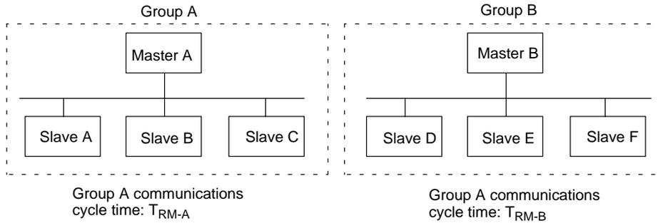
In Networks with two Masters, the communications cycle time for the entire Network will be the sum of the communications cycle times for the groups.
