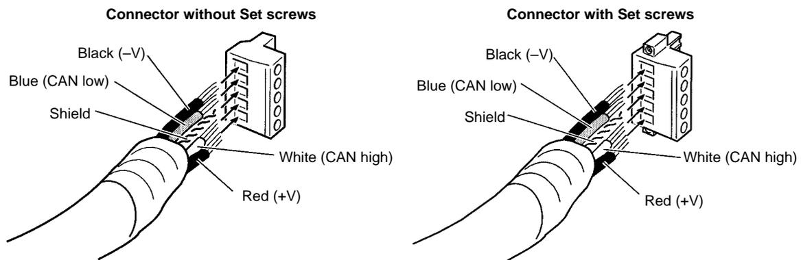
**Note** Be sure the line set screws are sufficiently loosened before attempting to insert the lines. If these screws are not loose, the lines will enter the gaps in the back of the connector and will not lock properly.
