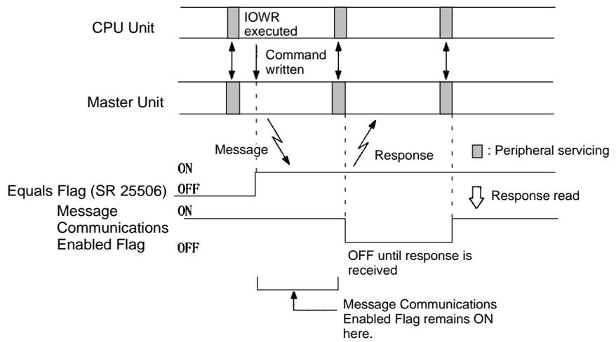
Use the type of programming shown below. The programming shown at the top will not always read the response properly.
