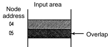
To eliminate the I/O area overlap and clear this error, change the node address setting on one of the Slaves as shown below and restart the Master by turning on the power again or restarting.
