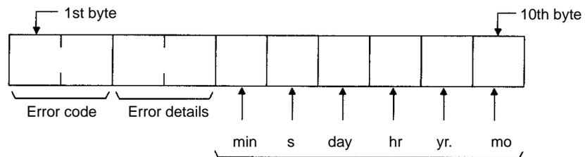
The time stamp is provided in the CVM1-DRM1-V1 Master Unit only. These bytes will be all zeros for the C200HW-DRM1-V1 Master Unit. (The program can be used to manually attach a time stamp to the error history records by using the clock in the CPU Unit for CS1-series and C200HX/HG/HE/HS PCs.)
