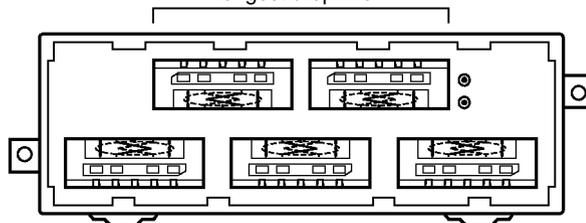
Align the cable connector with the socket on the T-branch Tap as shown in the following diagram and fully insert the connector into the socket. Tighten the set
