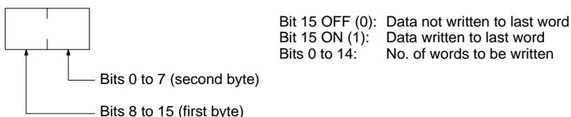
**Data (command):** The data to be written. The leftmost bits (bits 15 to 8) of each word must be specified first, followed by the rightmost bits (bits 7 to 0). The required number of bytes in total for each write can be calculated as follows:
