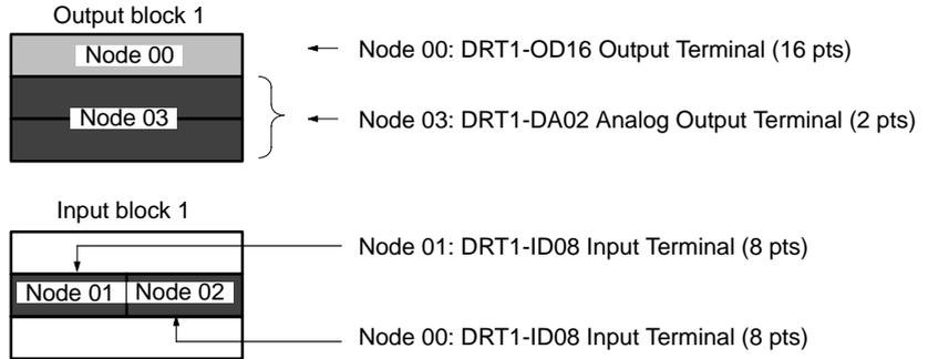
Each node address must be allocated at least one byte (rightmost or leftmost).
