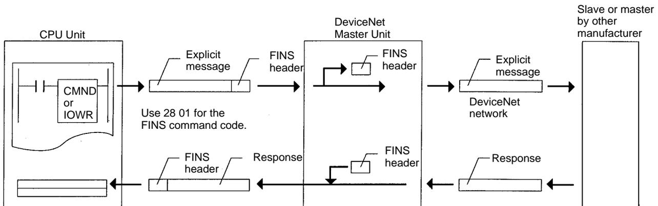
The local Master Unit is specified as the destination in the communications instruction in the PC's user program (not the OMRON Special Slave or Device-Net device made by another manufacturer), and the node address of the actual destination (i.e., the slave or master made by another manufacturer) is specified in the command data for the explicit message send command.
