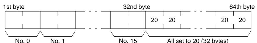
**Remote I/O data (response):** The number of remote I/O systems (SYSMAC BUS and SYSMAC BUS/2) is returned in two bytes as follows:
