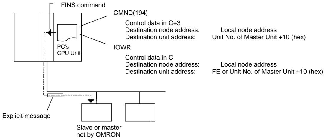
The following diagram shows an example of actual node address specifications.
