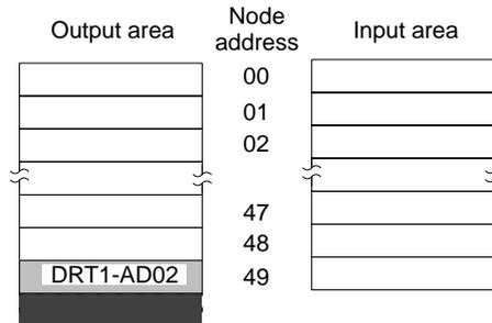
To eliminate the above problems and clear this error, change the node address setting on the Slave and restart the Master by turning on the power again or re-starting.
