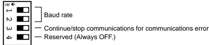
The settings of the DIP switch pins are shown in the following table. All pins are set to OFF at the factory.
