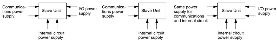
Because the power supplies for the communications, internal circuit and I/O are individually insulated as shown below, as a general rule each power supply should be connected separately.
