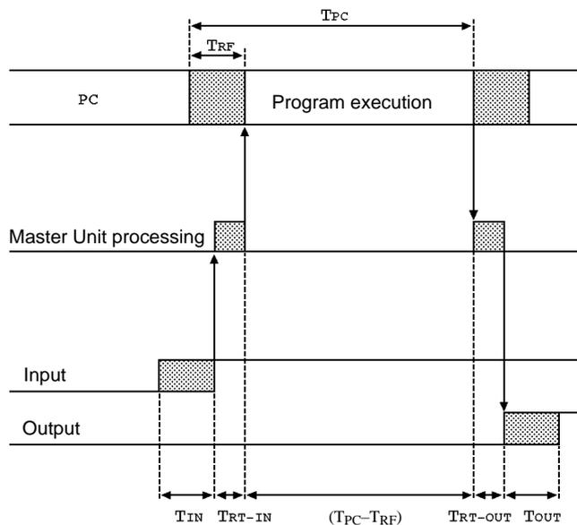
$T_{IN}$ : The Input Slave's ON (OFF) delay
