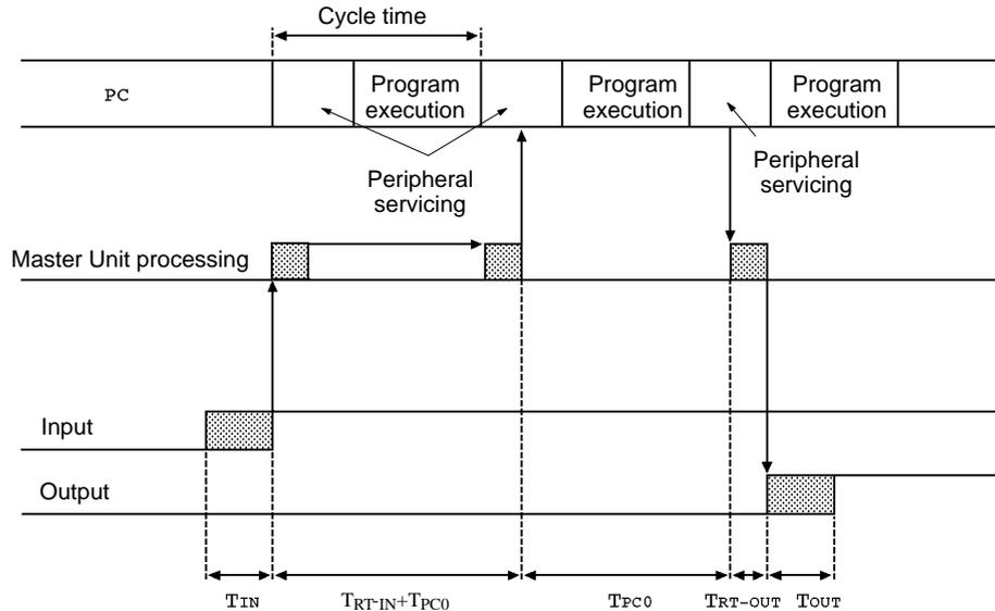
$T_{IN}$ : The Input Slave's ON (OFF) delay
