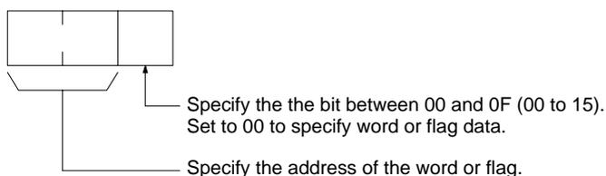
To obtain the corresponding address of the desired word or bit, add the data area word address (hexadecimal) to the first address of the range of addresses used for that data area in communications. For example, the address for word G134 is computed as follows:
