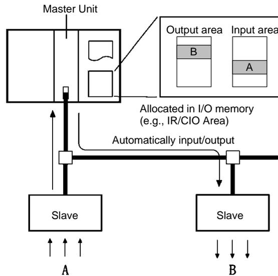
**Note** Input and output areas are automatically allocated in fixed areas unless a Configurator is used. A Configurator can be used to freely allocate input blocks 1 and 2, and output blocks 1 and 2, anywhere in I/O memory.
