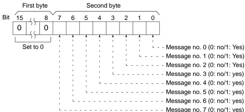
**FAL/FALS no. (response):** The highest priority FAL or FALS error. The actual value returned will be 4100 plus the FAL/FALS number; for details refer to the CV-series PC Operation Manual: Ladder Diagrams). If no FAL or FALS error has occurred, 0000 will be returned.
