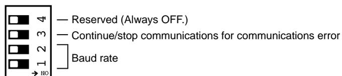
The settings of the DIP switch pins are shown in the following table. All pins are set to OFF at the factory.
