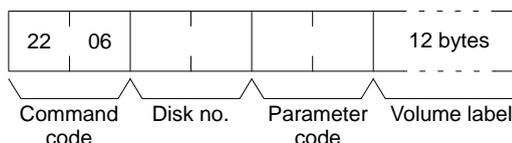
The command format for deleting a volume label is as follows:
