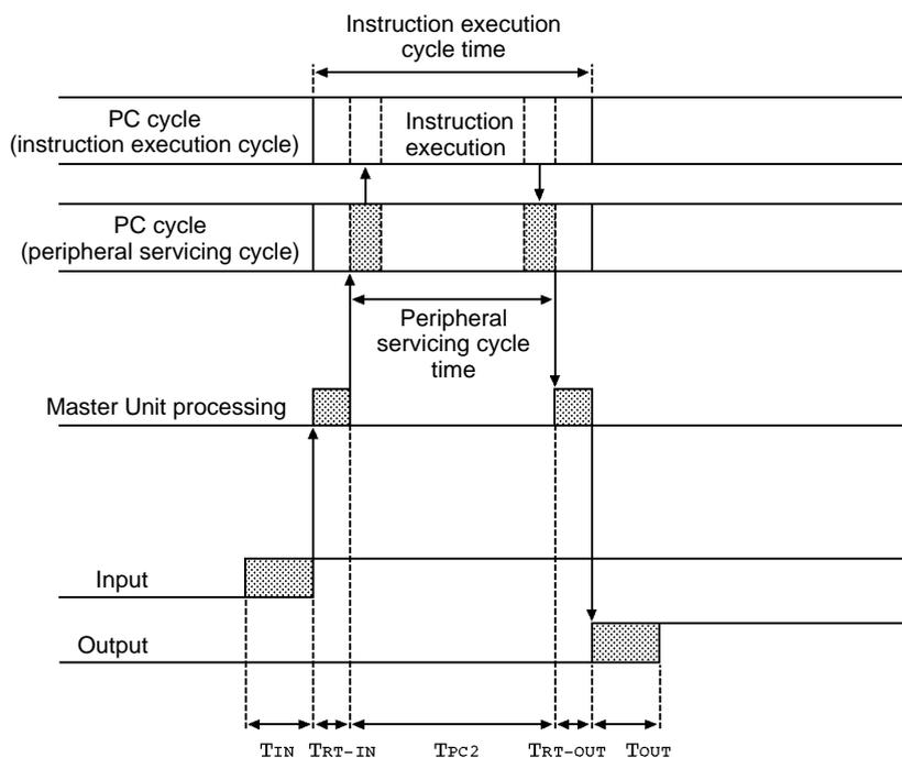
$T_{IN}$ : The Input Slave's ON (OFF) delay
