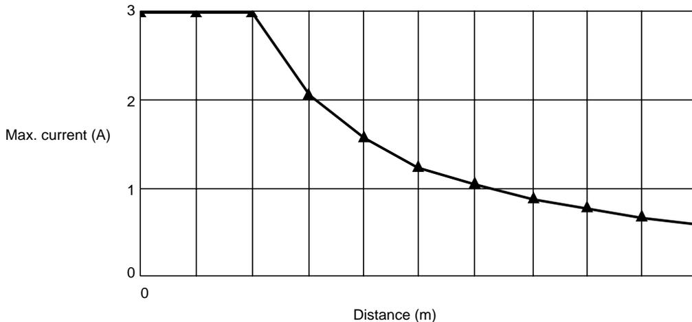
**6-4-1 Determining the Best Location of the Power Supply from a Graph**
