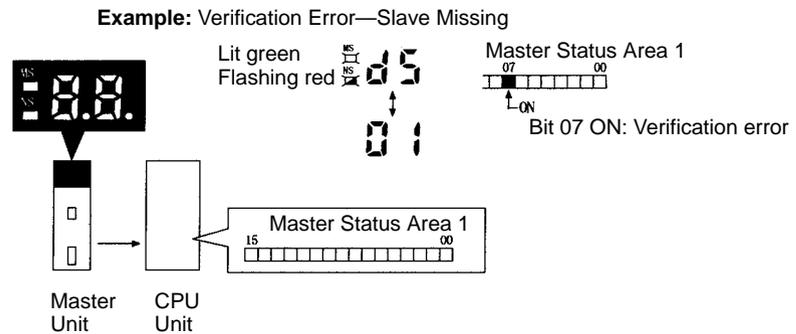
Each time a communications error occurs, an error code is placed in an error record in the error history kept in the RAM of the Master Unit. Up to 20 records can be stored in the error history. For CVM1/CV-series Master Units, the record is also time stamped. (Time stamps are not provided with the other Master Units.)
