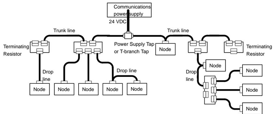
**Note** A node can be connected directly to the trunk line with the multi-drop method, but it is easier to connect a node to a drop line.
