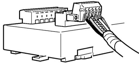
**Note** To avoid damaging the cable or breaking wires, don't pull on the cable or bend it too sharply when connecting it to the T-branch Tap. Also, never put heavy objects on top of the cable.
