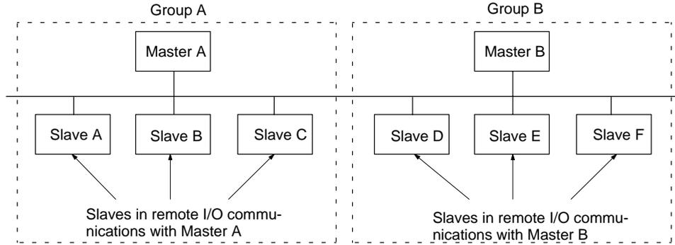
**Note** Although in the above diagram the Slaves are separated into two groups for convenience, the actual physical positions in the Network are irrelevant.
