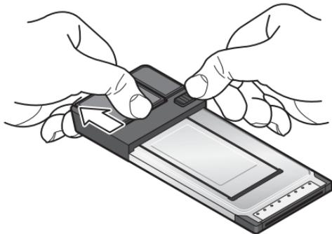
6. Gripping both sides of the device, insert it into your computer's ExpressCard slot (Sprint label facing up).
