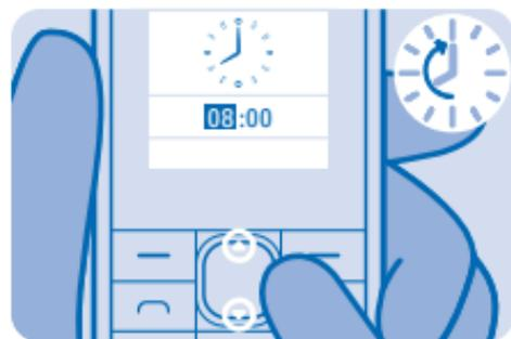
3. To set the hour, press up or down. To set the minutes, press right and then up or down. Press **OK**.
