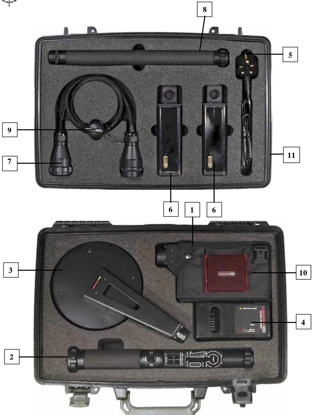
The TRANSIT CASE has a double safety lock. There is a pressure release valve positioned below the handle. Should the equipment have been subject to change in altitude or temperature the valve will automatically open.
