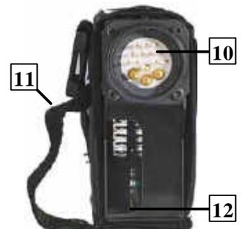
*The controls for the most commonly used functions such as receiver selection and range control, have been placed conveniently below the display screen. Selection via a unique 4-way thumb control.*
