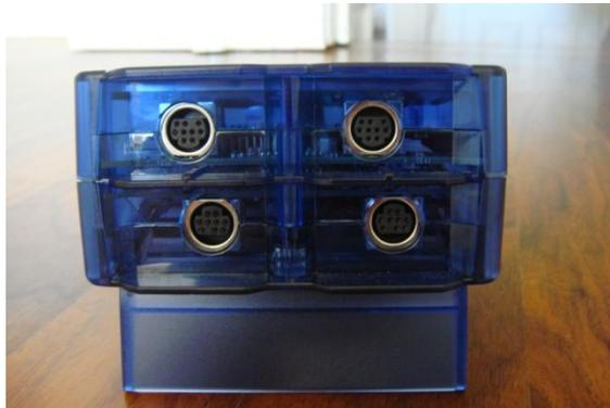
**Figure 1: Four Sensor Ports on top of GLX**
