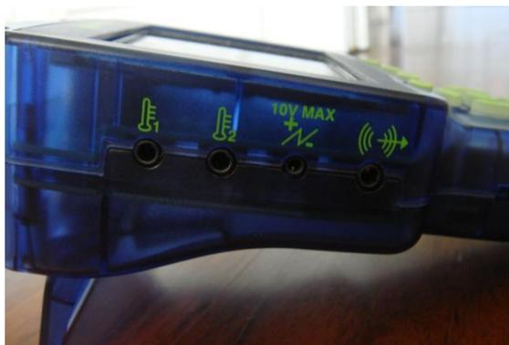
**Figure 2: Two Temperature Ports and Voltage Port on side of GLX**
