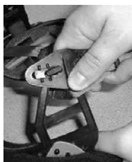
FIG. 10, FIG. 11 Headband Tab Repositioning
