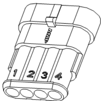
Fig. 7 Strela D232. Strela D485 connector and wiring
