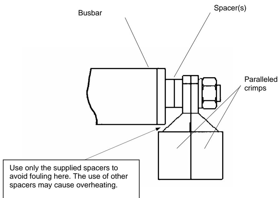
Figure 3-14 Use of spacers to avoid fouling busbar
