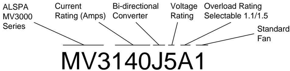
Figure 1-2 ALSPA MV3000eJ bi-directional converter identity code
