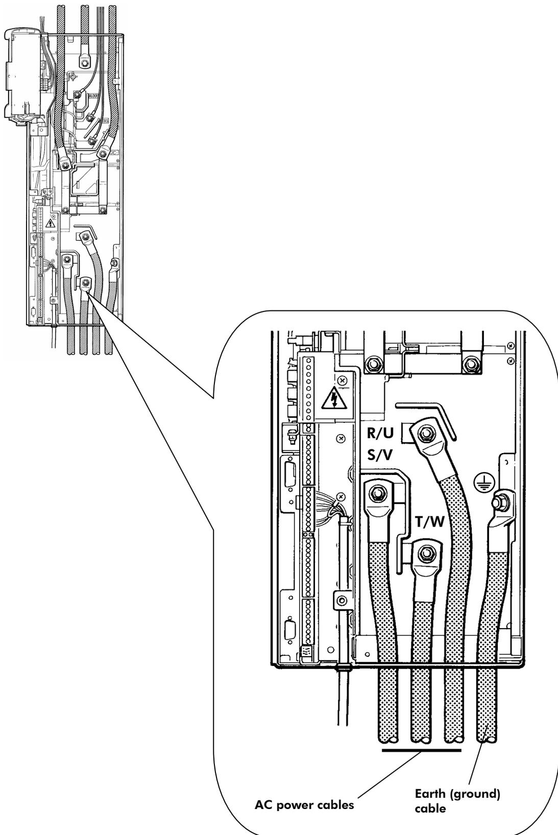
Figure 3-9 Power connections to frame sizes 3 and 4 (frame size 4 shown)
