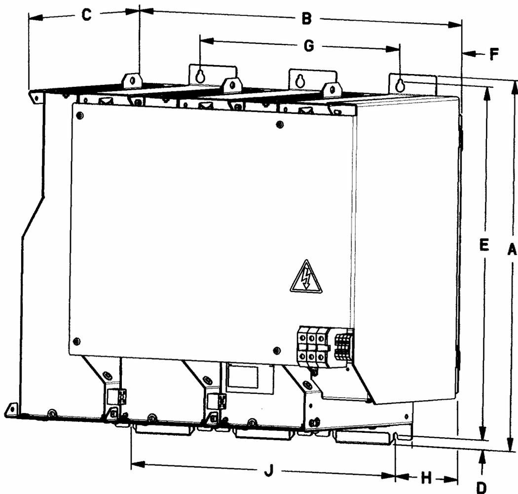
Figure 2-4 PWM filter for frame size 6 or 7 (size 7 shown)
