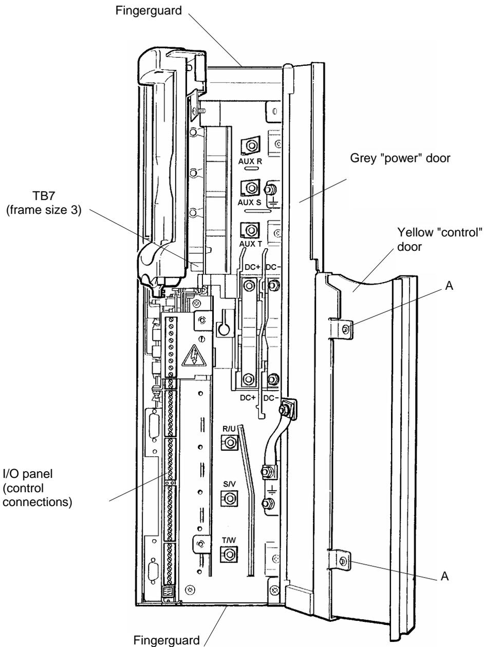
**Figure 3-7 Typical front view with doors open, showing electrical connectors (frame size 3 shown)**
