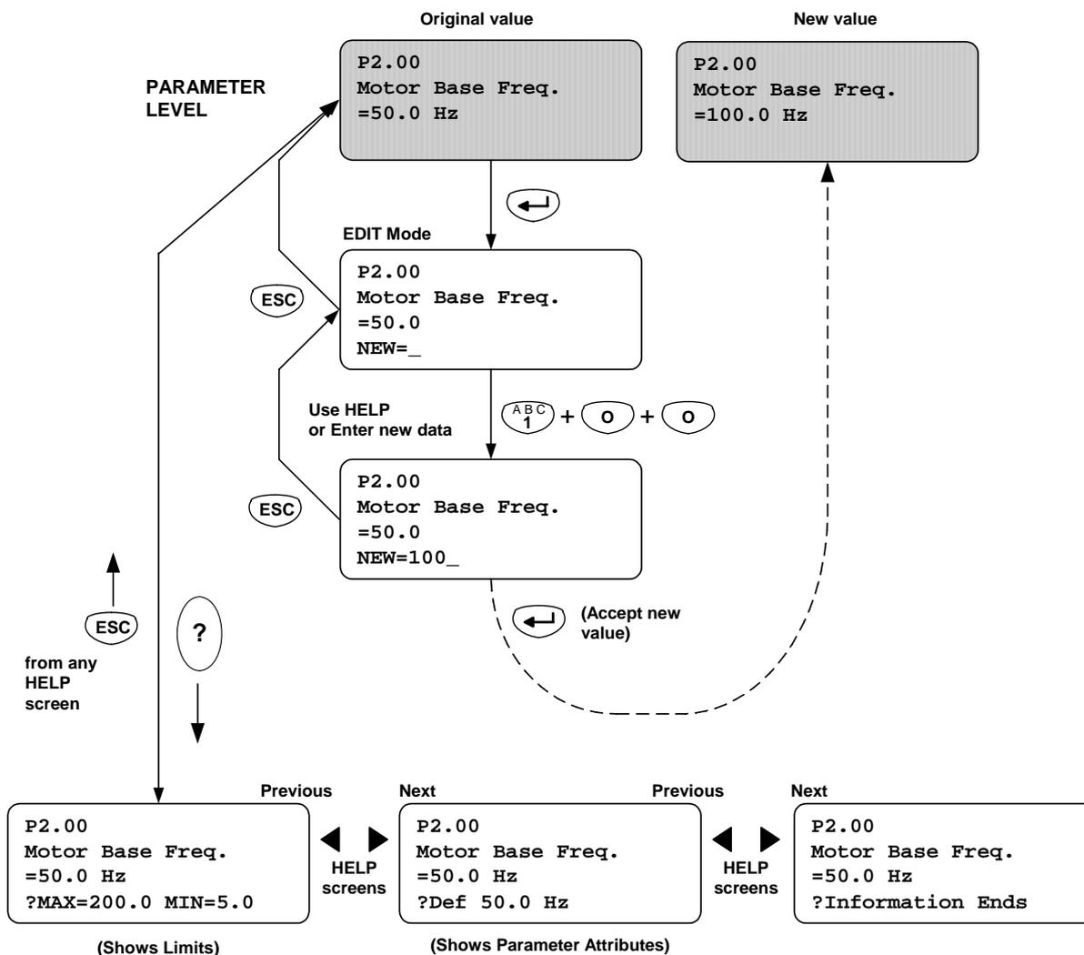
Figure 4-3 Editing a "numerical" parameter (example shows machine bridge)
