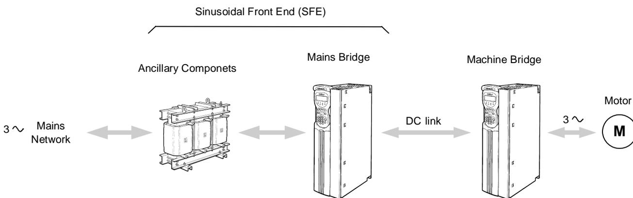
Figure 1-1 AEM Drive arrangement
