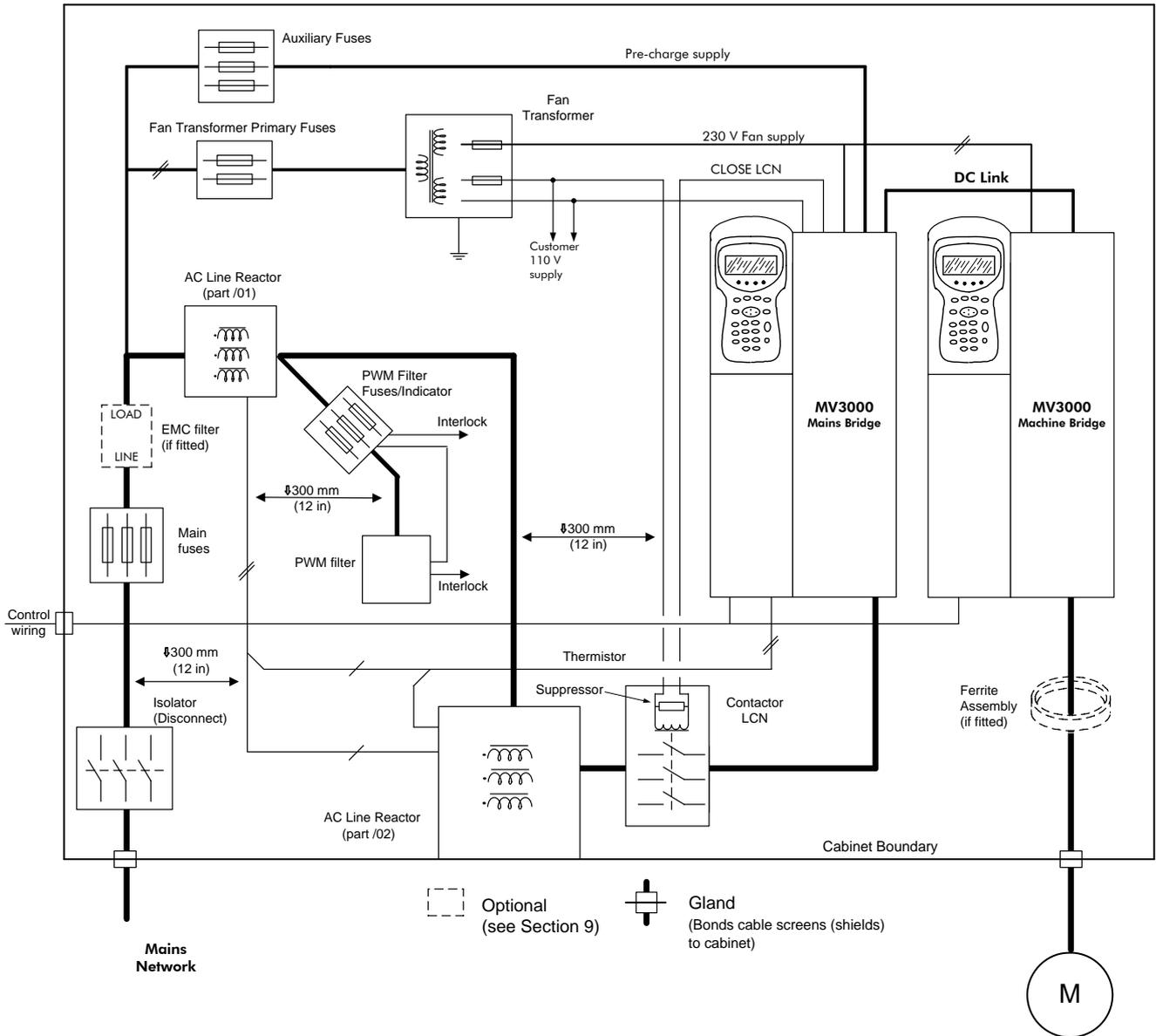
Figure 3-3 Typical cabinet layout for EMC compliance
