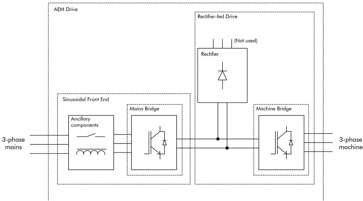
Figure 1-8 Simplified representation of an AEM drive using a SFE and a rectifier fed drive
