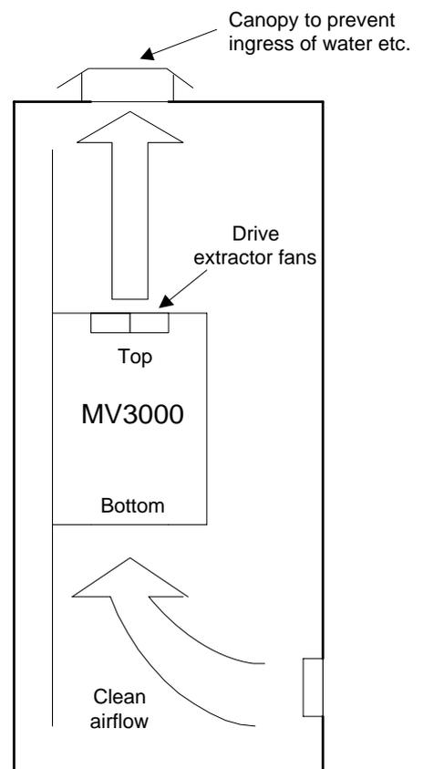
Figure 3-4 Typical airflow arrangement
