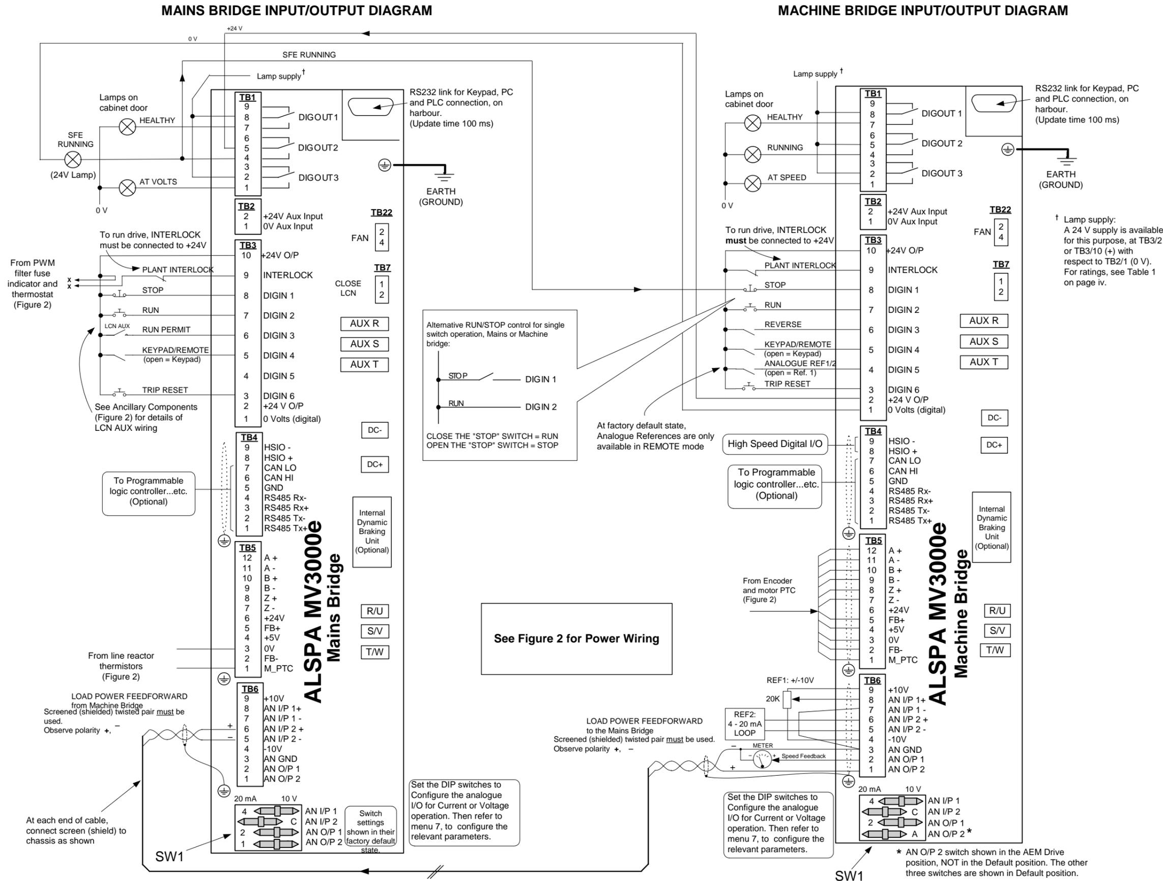
Figure 1 Bi-directional converter input/output diagram (default)
