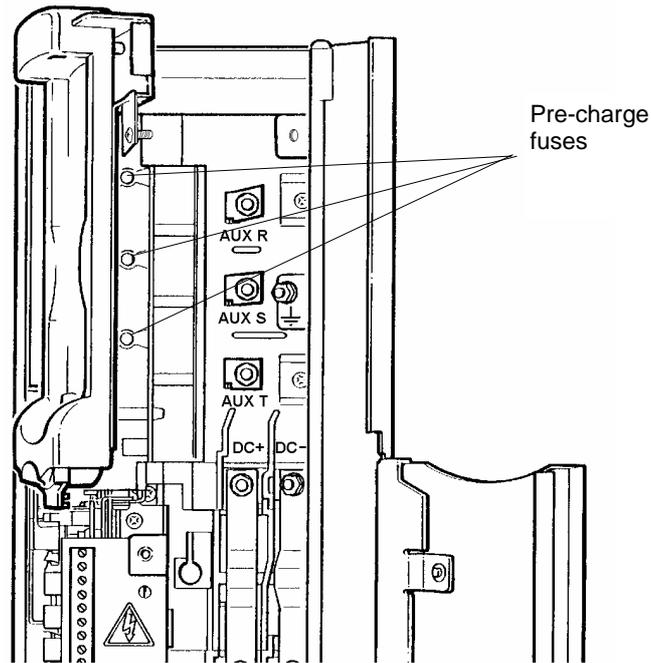
Figure 8-1 Frame size 3 and 4 pre-charge fuse access
