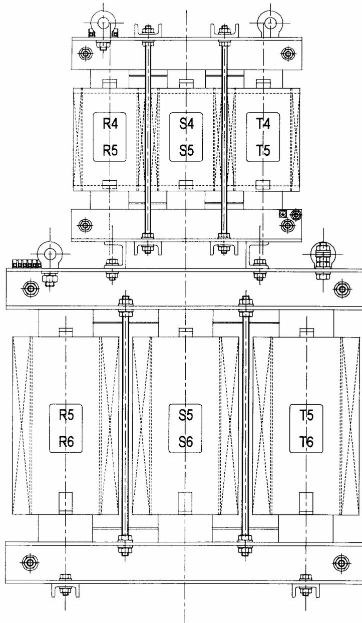
Figure 3-16 Illustration of stacked AC line reactors
