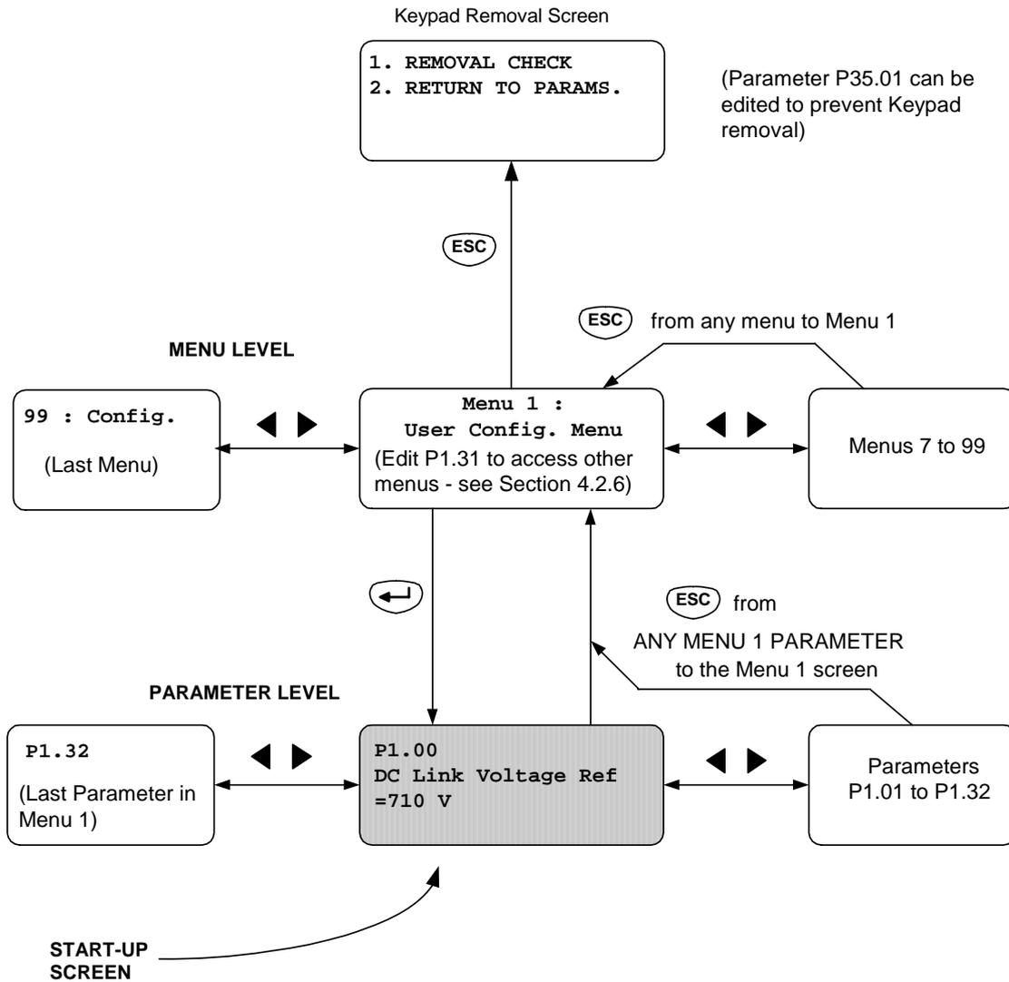
Figure 4-2 Navigating menus and parameters (example shows mains bridge)
