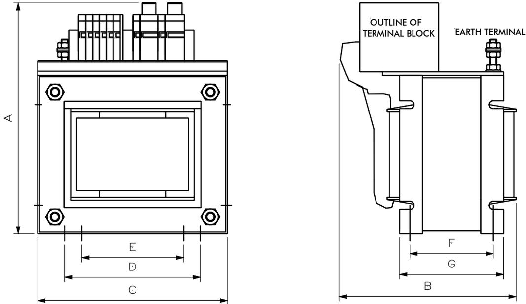
Figure 2-5 Fan transformer dimensions
