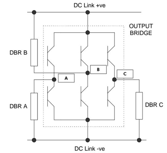
**Output Bridge Connections For Proportional DB Control**
