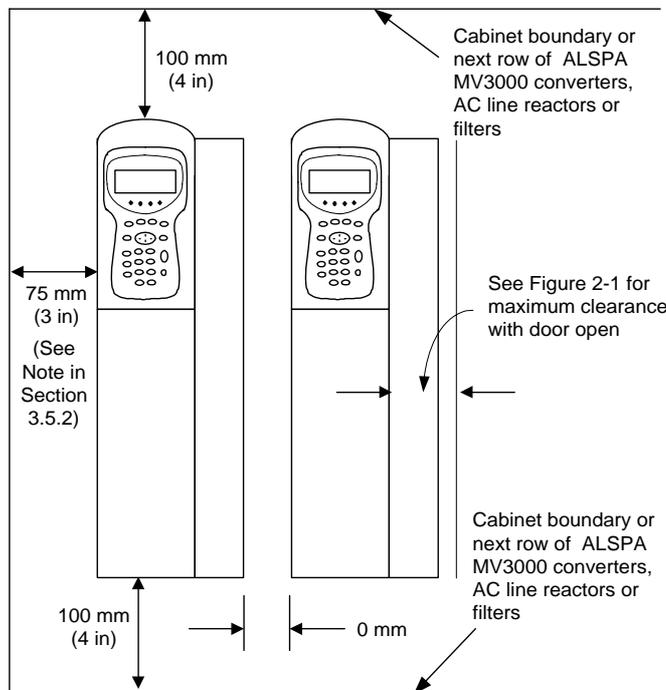
**Figure 3-5 Minimum recommended clearances**
