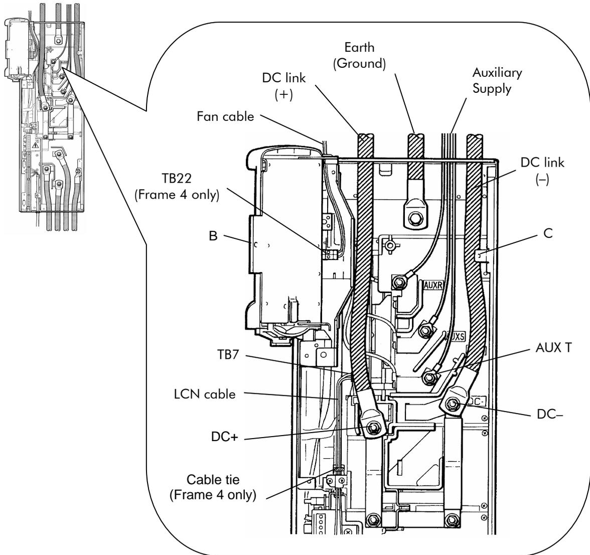
Figure 3-10 Ancillary wiring for frame sizes 3 and 4 (frame size 4 shown)
