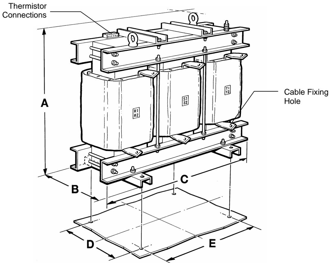
Figure 2-2 Line reactor (typical)
