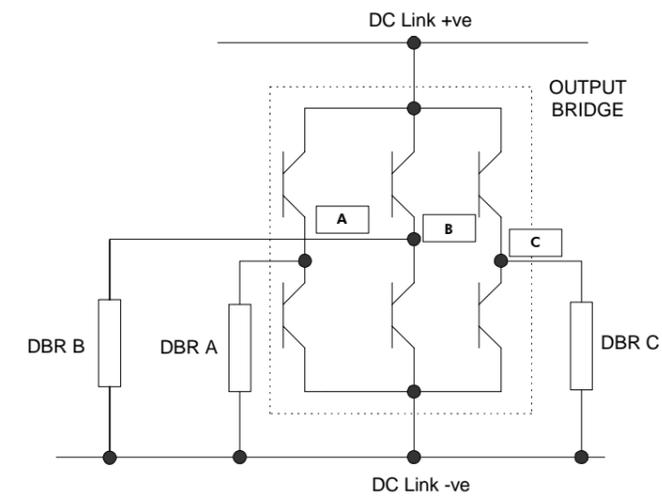
**Output Bridge Connections For Threshold DB Control**
