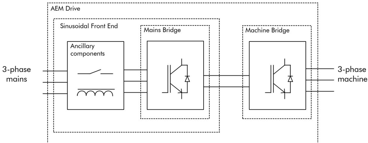
Figure 1-7 Simplified representation of an AEM drive using two identical bi-directional converters
