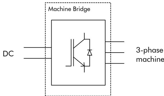
Figure 1-6 Simplified representation of a bi-directional converter configured as a machine bridge
