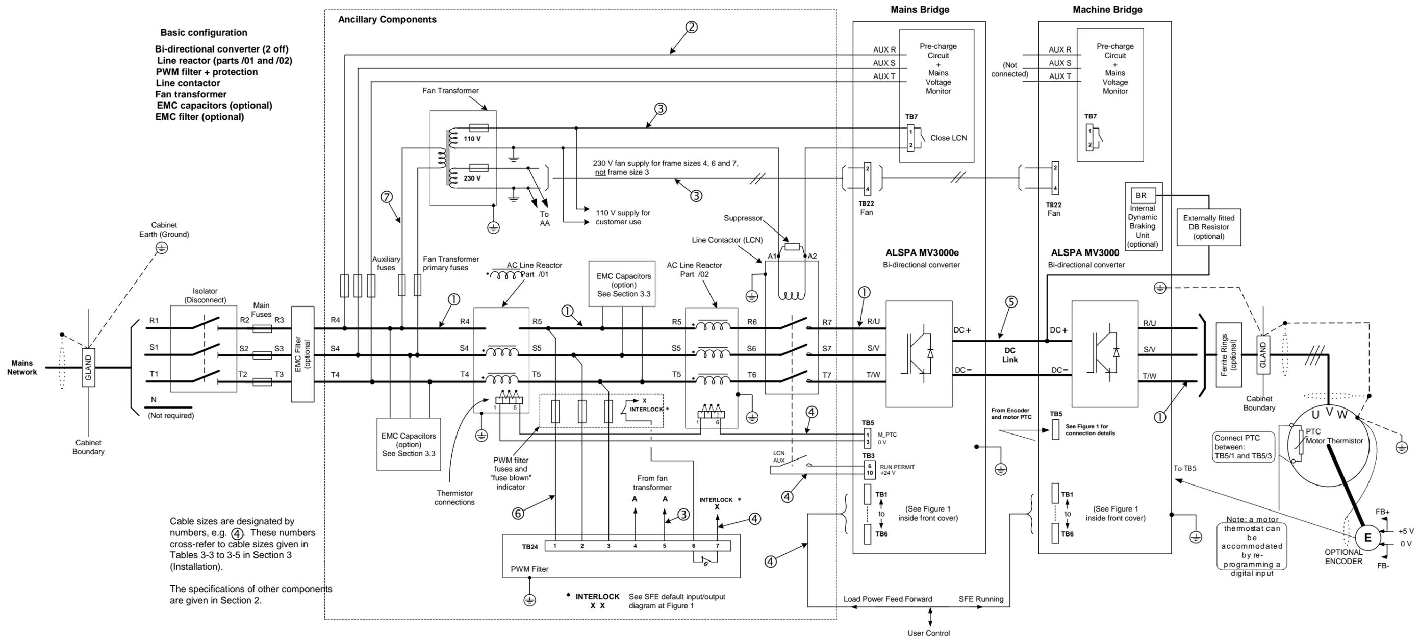
Figure 2 Interconnection diagram for an AEM drive
