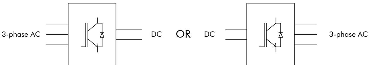
Figure 1-3 Simplified representation of a Bi-directional converter
