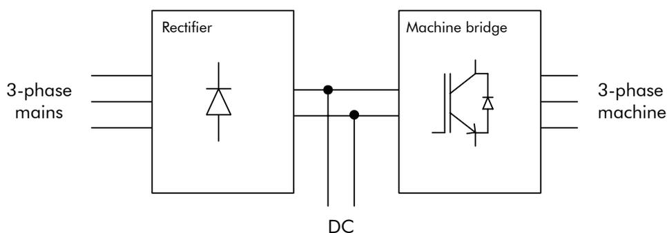
Figure 1-4 Simplified representation of a rectifier-fed drive
