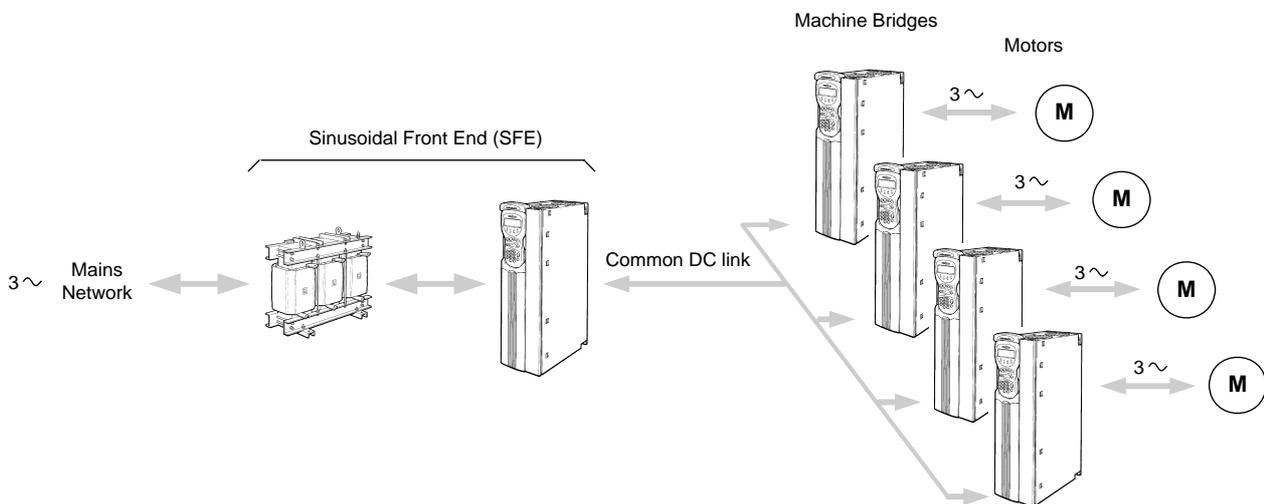
**Figure 1-9 Common DC link scheme with several machine bridges**
